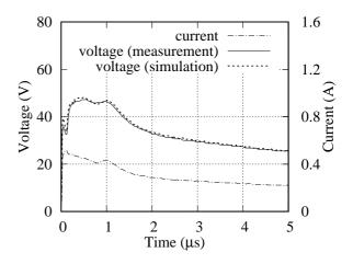
Figure 5: Measured and calculated ground potential rise.
