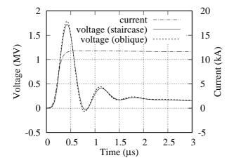
Figure 7: Top phase voltage corresponding to simulations with different wire models.
