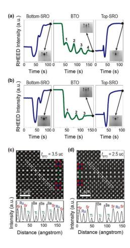
**Figure 1.** Time-dependent RHEED intensities for the growth of SRO/BTO/SRO heterostructures (a) with 3.5 uc-thick BTO layer and (b) with 2.5 uc-thick BTO layer. Insets are RHEED patterns of film surface taken along [100] azimuth. STEM-HAADF images of the SRO/BTO/SRO heterostructures with (c) 3.5 uc-thick BTO layer and (d) 2.5 uc-thick BTO layer along [100] zone axis. The following HAADF intensity profiles along the dashed boxes are also shown, respectively.
