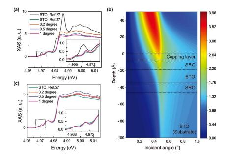
**Figure 3.** (a) Ti K-edge XAS of SRO/BTO/SRO heterostructure with  $t_{BTO} = 3.5$  uc on STO (001) for  $\pi$ polarized light with incident angles of 0.2, 0.5, and 1 degree. The reference XAS for bulk STO and BTO
