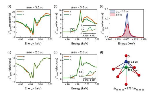
**Figure 5.** (a)[(b)] Real and (c)[(d)] imaginary part of atomic scattering factor of Ti in 3.5 uc (2.5 uc)-thick BTO layer. Ti scattering factor obtained from Ref. 36 is overlaid. (e) Intensities of Ti-K PEFS peaks for  $t_{BTO} = 3.5$  uc, and  $t_{BTO} = 2.5$  uc. (f) Schematic descriptions of ferroelectric distortions of TiO<sub>6</sub> octahedrons of 3.5 uc- and 2.5 uc-thick BTO layers.
