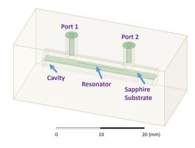
Figure 3: The cavity and resonator used in the HFSS simulation.
