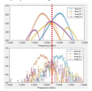
Figure 4: The real and imaginary compoents of the signal after the resonantor before adding the quantum noise (Top) and after the amplification chain in Fig. 1 (Bottom). The red dotted line indicates the reading pulse frequency.
