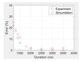
Figure 7: Simulated and meaasured readout errors of the qubit readout system as a function of readout pulse duration.
