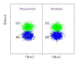
Figure 8: The quadrature measurement (Left) and simulation (Right) for reading  $|0\rangle$  and  $1\rangle$  states, with a readout pulse power 8dB less than the nominal power and  $t_p = 3.5 \mu s$
