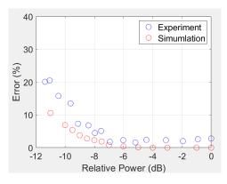
Figure 9: Simulated and measured readout errors of the qubit readout system as a function of readout pulse power relative to the nominal power.
