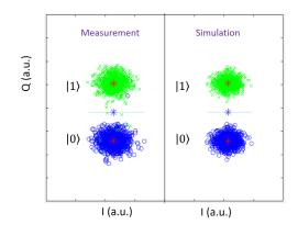
Figure 5: The quadrature measurement (Left) and simulation (Right) for reading  $|0\rangle$  and  $1\rangle$  states, with readout pulse at nominal power and  $t_p = 3.5 \mu s$
