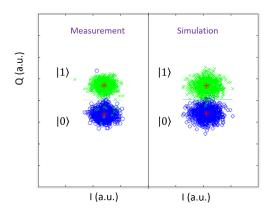
Figure 6: The quadrature measurement (Left) and simulation (Right) for reading  $|0\rangle$  and  $1\rangle$  states, with nominal readout power and  $t_p = 2.0 \mu s$
