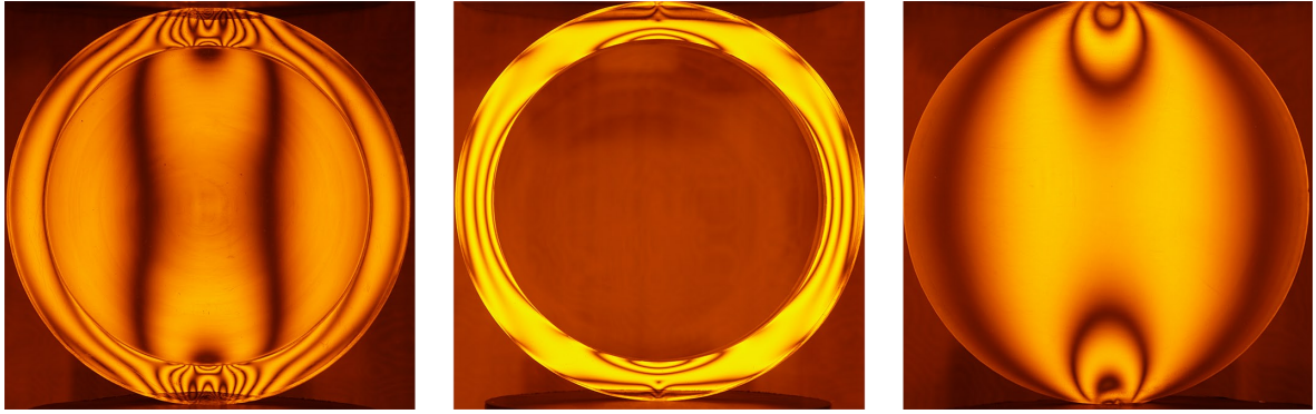
Figure 6: Monochromatic photoelastic fringes under diametrical compression of: a coated disk (left), its external ring (center), and the inner disk without coating (right). Samples are shown in Fig. 5 (upper part).
