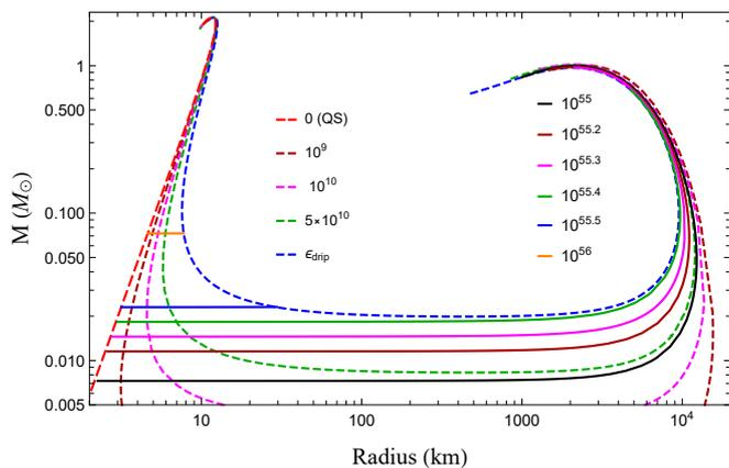
**Fig. 1.** MR sequences. Dashed lines show configurations in which  $P_t$  is constant. By increasing  $P_0$  (and therefore also  $B_{\text{core}}$ ) the curves are followed clockwise. The legend indicates  $\varepsilon_t$  values in  $\text{g}/\text{cm}^3$ . Solid lines show configurations in which  $B_{\text{core}}$  is constant. Here, by increasing  $P_0$  (and therefore also  $P_t$ ) the curves are followed anti-clockwise. The legend indicates the value of  $B_{\text{core}}$ .
