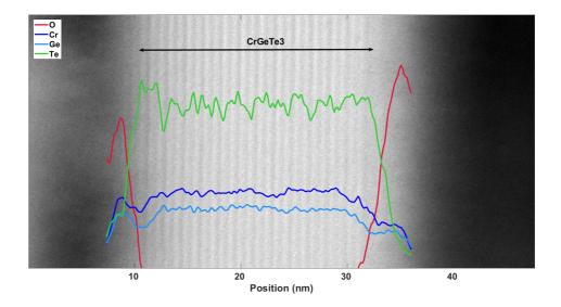
**Supplementary Figure S5.** EDS line scan, showing the relative amount of Cr, Ge, Te and O in a cross section of the device, in arbitrary units. The results are superimposed on a high-angle annular dark field (HAADF) image of the same cross section.
