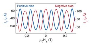
Supplementary Figure S1. Quantum interference pattern of the SQUID-on-tip (SOT). The critical current  $I_c$  of one of the SOT's used in this work as a function of the applied out-of-Plane field  $H_z$ . Blue: Positive bias, red: Negative bias. The period of 105 mT of the quantum interference corresponds to an effective diameter of 155 nm of the SOT.
