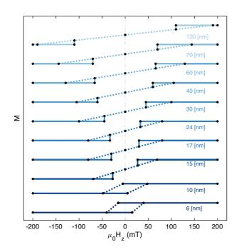
Supplementary Figure S3. Transport of bilayer CGT/NbSe<sub>2</sub> at different thickness at 4.2 K. Sketched magnetization curves drawn from  $B_z(x, y)$  measured on film's parts of different d. Dashed lines are a guide to the eye connecting the two saturated fields. Thickness from bottom to top d = 6, 10, 15, 17, 24, 30, 40, 60, 70, 130 nm
