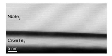
**Supplementary Figure S4.** High angle annular dark-HAADF image of the heterostructure in the sacrificial device where layers of CGT are seen to be separated by a gap from layers of NbSe<sub>2</sub>.
