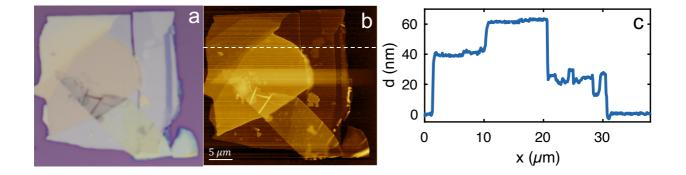
**Supplementary Figure S2.** AFM and optical thickness characterization. (a) Optical image of an exfoliated CGT flake on a SiO<sub>2</sub> substrate. The CGT flake contains varying thicknesses with correlated colors ranging from light purple (thinnest) to yellow (thickest). (b) A topography image of the flake seen in panel a, taken by an AFM using the tapping mode. (c) A topography cross section taken along the dashed line in panel b, sowing areas with distinct (uniform) thicknesses.
