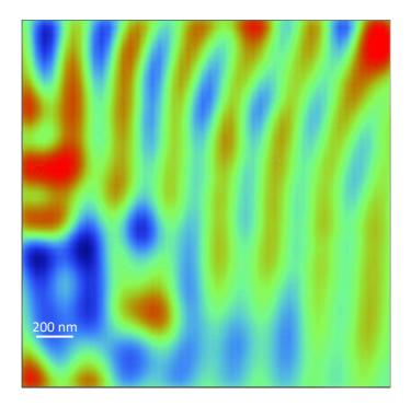
Supplementary Figure S7. SQUID-on-tip image of 130 nm CrGeTe3 after zero field cooling (SOT). Stripe magnetization with zero net magnetization in agreement with the theoretical prediction in the limit where the dipolar interaction exceeds the magnetic anisotropy. area scan  $2x2 \ \mu m^2$ , pixel size 52 nm. The blue to red color scale represents lower and higher magnetic field respectively.
