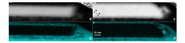
Supplementary Figure S10. EDX and STEM of 17 and 24 nm flake edges. (a-b) STEM cross-sectional images measured on the black lines presented in Fig. 4 c,d. (c-d) EDX measurements of the same cross-sections showing similar levels of oxidation on the edge and surface.
