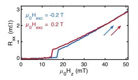
Supplementary Figure S11.  $R_{xx}$  magneto-transport measurements of bilayer CrGeTe<sub>3</sub>/NbSe<sub>2</sub> showing magnetic memory at  $\mu_0 H_z = 0$  for CGT of thickness d < 10 nm.  $R_{xx}$  as a function of the out-of-plane (OOP) field  $H_z$  from zero to above the saturation field  $H_s$  after different excursions at  $\mu_0 H_{ex} = -0.2$  T and  $\mu_0 H_{ex} = +0.2$  T, blue and red curves, respectively.
