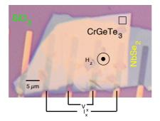
**Supplementary Figure 6.** Optical image of the bilayer and the Au electrodes used for the transport measurements presented in figure 1 and 2 of the main text. The black square corresponds to the region image in Fig. 1 b-g and Fig. 2. c-j of the main text.
