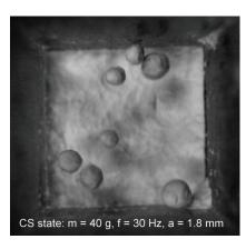
FIG. 11. Agglomerates on the top free surfaces of the consolidated powder bed. This image corresponds to the top view of the Fig. 2(c) in this paper.
