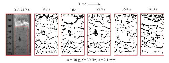
FIG. 9. Static fracturing (SF) phase. ImageJ [22] is used to observe the deformations in the bulk. The cracks/voids present in the bulk keep deforming to form elongated horizontal cracks. The experimental conditions are m = 30 g, f = 30 Hz, and a = 2.1 mm.
