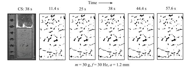
FIG. 8. Consolidated (CS) phase. ImageJ [22] is used to observe deformations in the bulk. During CS phase, we do not observe any deforming voids. The experimental conditions are m = 30 g, f = 30 Hz, and a = 1.2 mm.
