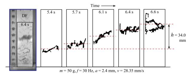
FIG. 5. Decompaction-wave propagation in DF regime. ImageJ [22] was used to track cracks in the bulk. The red dashed lines represent mean locations of the cracks. The standard deviation about mean of the data is defined here as a crack width w.
