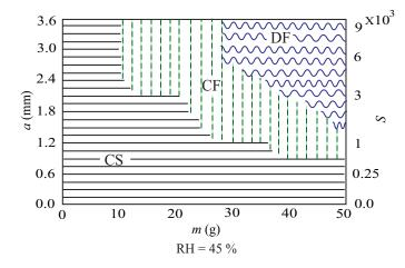
FIG. 13. The Phase diagram for a powder with mean diameter size  $d = 18 \ \mu \text{m}$  at  $f = 30 \ \text{Hz}$  and RH = 45%. The regime CF represents convective fracture (shown by vertical green dashed lines).
