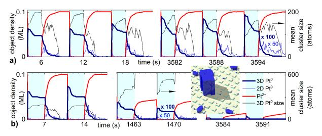
Figure 7: KMC simulations of stable (a) and unstable (b) nanoparticle populations during alternating oxidizing/reducing conditions. Step density 17% ML, Pt amount 10% ML. Cycle times: (a) 2 s reduction, 4 s oxidation (b) 3 s reduction, 4 s oxidation. Reduction cycles are highlighted light blue. Inset in (b): KMC morphology at 1470 s.
