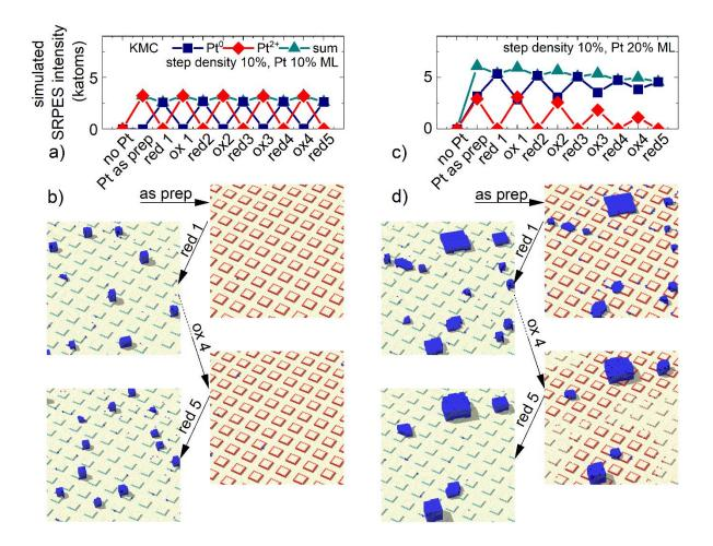
Figure 5: KMC simulation of redispersion and coarsening of Pt load. Redispersion and coarsening are induced by alternatingly switching the step edges from oxidized to reduced. Step density 10% ML, Pt amount (a), (b) 10% ML, (c), (d) 20% ML. (a), (c) Single atom  $(Pt^{2+})$ , metallic  $(Pt^{0})$ , and Pt total ("sum") simulated SRPES signal. (b), (d) KMC morphologies. Color coding: red - Pt<sup>2+</sup> ions, blue - metallic Pt, pink - oxidized step, cyan - reduced step.
