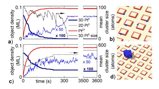
Figure 6: KMC simulations of stable (a, b) and unstable (c, d) nanoparticle populations upon redispersion of 3D Pt clusters at stationary oxidizing conditions. Step density 10% ML, Pt amount (a, b)  $(10+\varepsilon)$  % ML,  $\varepsilon=0.15$  % ML, (c, d) 15 % ML. (a, c) time evolution of density of Pt<sup>2+</sup> single atoms, subcritical 2D Pt<sup>0</sup> clusters, 3D Pt<sup>0</sup> clusters, and average 3D Pt<sup>0</sup> cluster size. (b, d) KMC morphologies at 3600 s.
