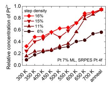
**Figure 1: Redispersion of Pt deposited on CeO<sub>2</sub>(111) in UHV.** Pt was deposited at 300 K and flash annealed in UHV to increasingly higher temperatures. The final step of the thermal treatment is annealing in UHV at 700 K for 5 min.
