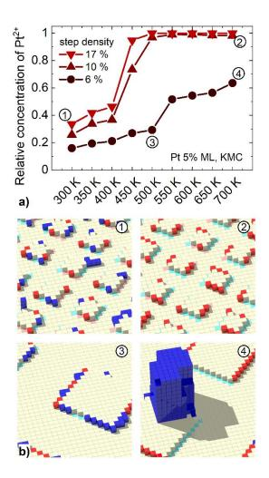
**Figure 4: KMC simulation of Pt redispersion in single-atom traps.** a) Pt deposition at 300 K and intermittent annealing to increasingly higher temperatures. b) KMC morphologies corresponding to the points ①-④ in a). Color coding: red - Pt<sup>2+</sup> ions, blue - metallic Pt, pink - oxidized step, cyan - reduced step.
