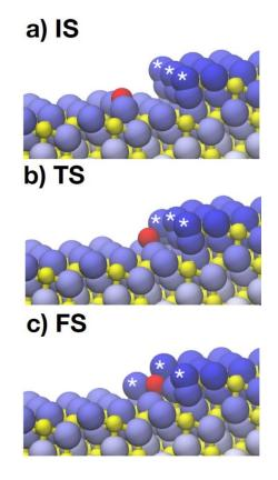
**Figure 3. Representative configurations of the calculated minimum energy path for the Pt adatom diffusion and incorporation at Type II Excess Oxygen step edge.** Panels a-c displays the initial (IS), transition (TS) and final (FS) states of the process. Pt atom red, Ce atoms yellow, O atoms blue. Excess O atoms are indicated with \*.
