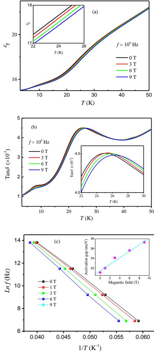
Fig. 5. (a) The temperature dependence of dielectric permittivity  $\epsilon_r$ , and (b) dielectric loss  $\tan\delta$  under different magnetic field and fixed  $f = 10^6$  Hz for  $\text{Ba}_9\text{Fe}_3\text{Se}_{15}$ . The insets of (a) and (b) show their enlarged view, respectively. (c) The relationship between  $\ln f$  and the peak temperature of  $\tan\delta$  for different magnetic field. The inset is the activation energy gap versus magnetic field.
