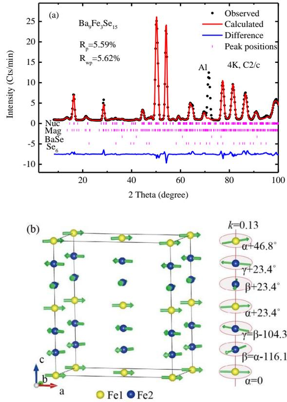
Fig. 2 (a) The Rietveld-fit of the magnetic intensities measured by powder neutron diffraction by the HB-3 Spectrometer ( $\lambda = 2.3579 \text{ \AA}$ ) at 4 K for  $\text{Ba}_9\text{Fe}_3\text{Se}_{15}$  sample. (b) The sketch of the magnetic structure, showing a spin spiral configuration.
