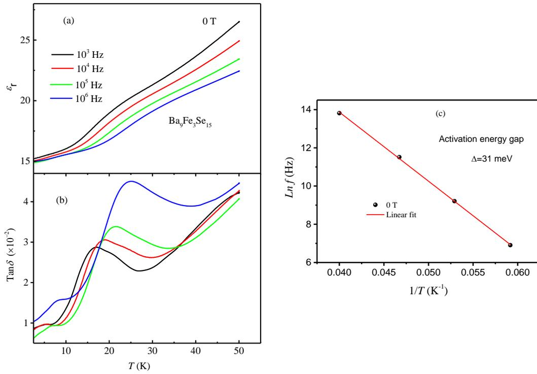
Fig. 4. (a) The temperature dependence of dielectric permittivity  $\epsilon_r$ , and (b) dielectric loss  $\text{tan}\delta$  under different frequencies and zero magnetic field for  $\text{Ba}_9\text{Fe}_3\text{Se}_{15}$ . (c) The relationship between the frequency and the inverse temperature of the dielectric loss peak. The red line is the linear fit.
