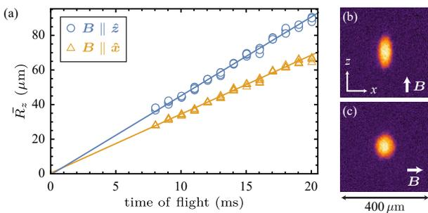
FIG. 2. (a) Measured dependence of the rescaled condensate radius  $\bar{R}_z$  on the time of flight. The blue open circle (yellow open triangle) is measured  $\bar{R}_z$  when the magnetic field is set parallel to the  $z$  ( $x$ ) axis. The solid line is the linear fit to the data. Typical absorption images after 20 ms-long time of flight are shown in (b) and (c), where the magnetic field is set parallel to the  $z$  and  $x$  axes, respectively.
