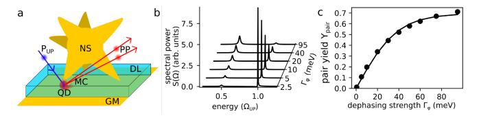
FIG. 2. Dephasing induced degenerate down-conversion in an USC system. a) Schematic of a possible realization of the proposed single-photon parametric down-conversion scheme. A gold nano-star (NS) placed on a gold mirror providing a mirror charge (MC) and separated by a few nm thick
