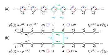
FIG. 1. Schematic of the CROW with two embedded resonators. (a) 1D coupled resonator array. The black dots in the central two resonators in green are the scatterers, which induce the intra-resonator intermodal couplings -s in cyan. (b) Schematic of the quasi-1D tight-binding model of (a). The upper (lower) lead represents the CW (CCW) mode of the resonator array. The steady-state wave functions are marked.
