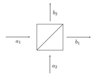
FIG. 1. Schematic representation of a beam splitter. In the classical theory, input modes with complex amplitudes  $a_1$  and  $a_2$  are superposed to form the output amplitudes  $b_1$  and  $b_2$ . In the quantum theory these complex amplitudes are replaced by photon annihilation operators.
