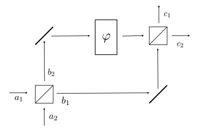
FIG. 2. Schematic representation of a Mach-Zehnder interferometer. The input beam splitter is as in Figure 1 with transmission and reflection coefficients  $t_1$  and  $r_1$ . The lengths of the two arms are  $L_1$  and  $L_2$ so that propagation along the arms produces the phase shifts  $kL_1$  and  $kL_2$ . For completeness, we include, also an additional element in the upper arm producing an additional phase shift  $\varphi$ .
