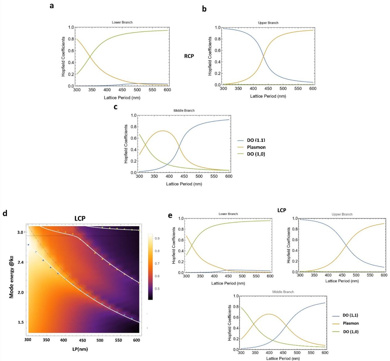
Figure S5. Hopfield coefficients calculated from RCP extinction maps for the lower (a), upper (b), and middle (c) branches. d) Extinction dispersion at normal incidence for left-handed circularly polarized light in water environment obtained from numerical simulations. e) Hopfield coefficients for LCP retrieved from the simulated extinction dispersion.
