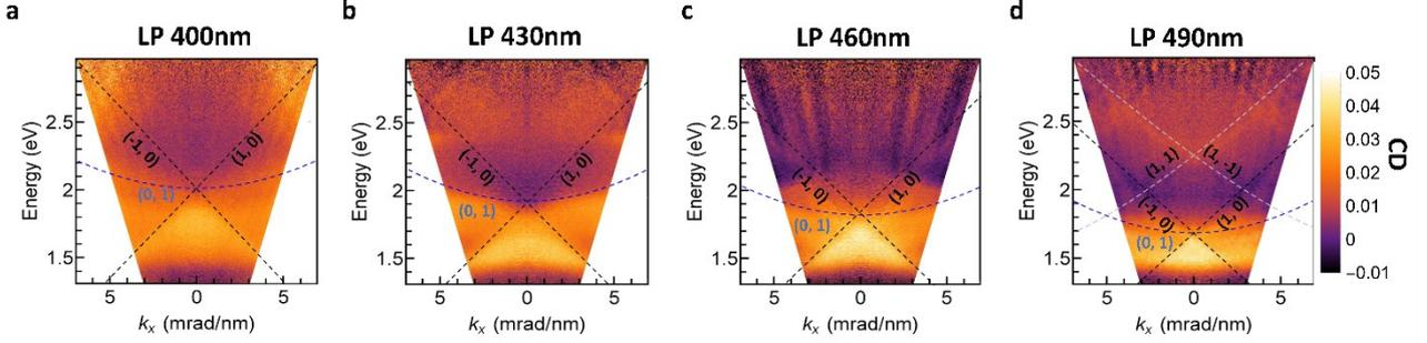
Figure 2. Energy-momentum experimental CD extinction maps defined as the difference between measured LCP and RCP extinction (shown in figure S3) at different LPs (400 nm, 430 nm, 460 nm, 490 nm). The dashed lines are drawn to highlight the progressive DO dispersion shift when increasing LP. The dispersion of the DOs were calculated from eq. 1 for the indicated ( $N_x, N_y$ ) indices.
