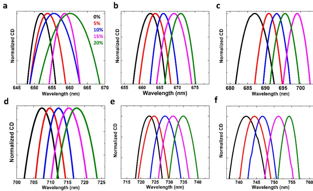
Figure S7 a-f. CD spectra of the NH arrays as a function of the surrounding refractive index environment (0%, 5%, 10%, 15% 20% of glycerol in water solution), zoomed at the relative resonance peaks measured for different lattice periods: a) LP 370nm, b) LP 400nm, c) LP 430nm, d) LP 460nm, e) c) LP 490nm, f) LP 520nm.
