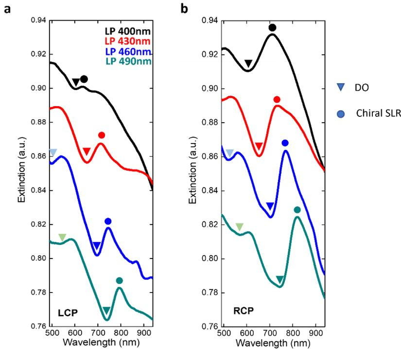
Figure S2. a-b. LCP and RCP extinction spectra recorded for arrays of  $30 \times 30$  elements and with different LPs in oil environment. The maxima are attributed to the c-SLRs spectral peaks (indicated by the circles), while the dips indicate the diffractive  $(\pm 1, 0)$  DOs (represented by the triangle). In the arrays with LP=460nm and LP=490nm, the lightest triangles indicate the  $(\pm 1, \pm 1)$  DOs.
