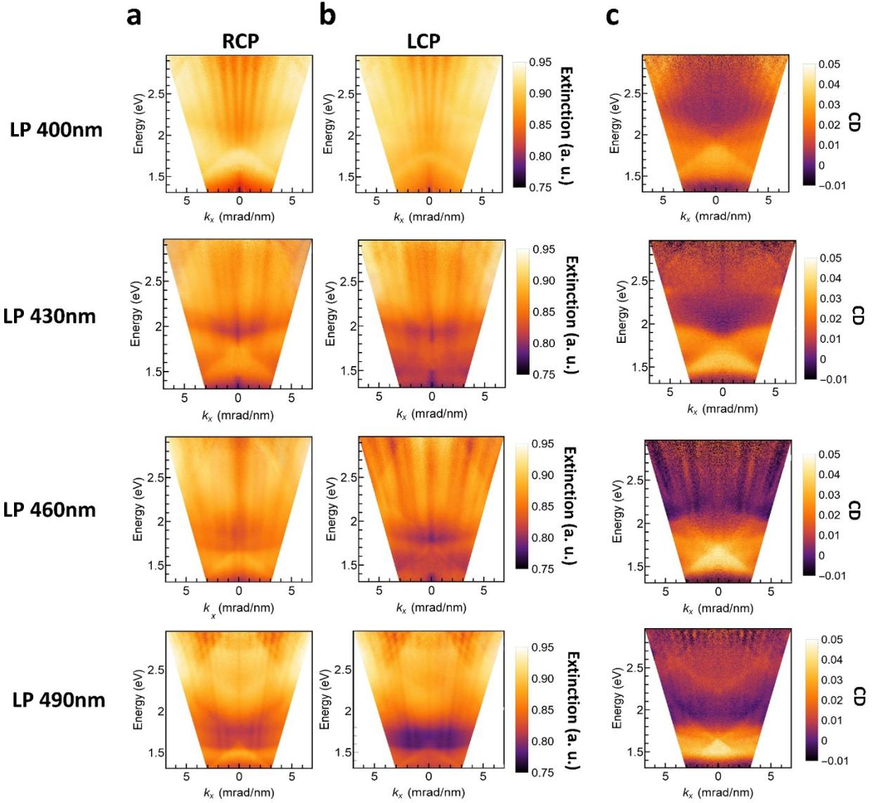
Figure S3. a-b. Experimentally measured energy-momentum extinction dispersions for LCP and RCP light for four different lattice periods (400 nm, 430 nm, 460 nm, 490 nm). c. Circular dichroism far-field maps as a function of LP calculated as the difference between RCP and LCP extinctions.
