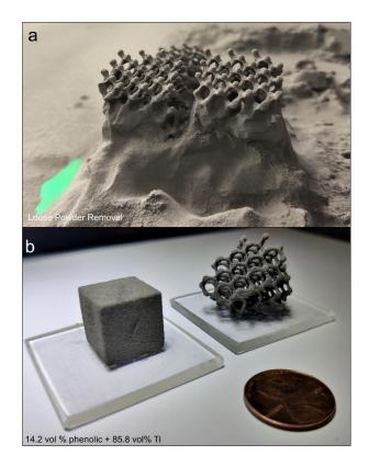
**Figure 3.** Green components formed from 14.2 vol% phenolic resin powder + 85.8 vol% Ti during removal from the powder bed (a) and after loose powder was removed (b). The structures shown in (b) had low interparticle binding leading to damaged features and disintegration of the cube and lattice corners when handled.
