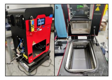
**Figure 1.** (a) Sinterit Lisa Pro® selective laser sintering machine modified for compatibility with variable argon flow. (b) Photograph of the interior of the build chamber containing precursor powder.
