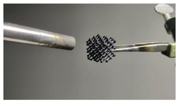
Figure 13.Video demonstration of  $TiC_x$  lattice (fabricated by post-processing using Scheme II) that was heated using a propane torch.
