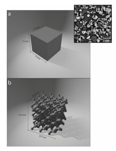
**Figure 2.** Digital representation of the printed test structures: (a) 15 mm x 15 mm x 15 mm cube and (b) diamond lattice structure. (c) shows a BSE-SEM micrograph of the 75/25 vol% Ti/phenolic precursor particle morphology, where large bright particles are Ti, and dark particles are phenolic.
