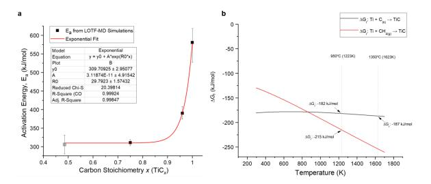
**Figure 12.** (a) The influence of carbon content on the activation energy required for C diffusion in  $TiC_s$ . The lower data point for  $TiC_{0.48}$  was reported in [45]. (b) The temperature-dependent  $\Delta G_r$  associated with Ti reaction with  $C_s$  or CH<sub>4</sub>.
