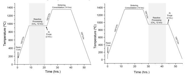
**Figure 5.** Heating schedules for reaction conversion of 75 vol% Ti + 25 vol% phenolic green state parts to TiC components.
