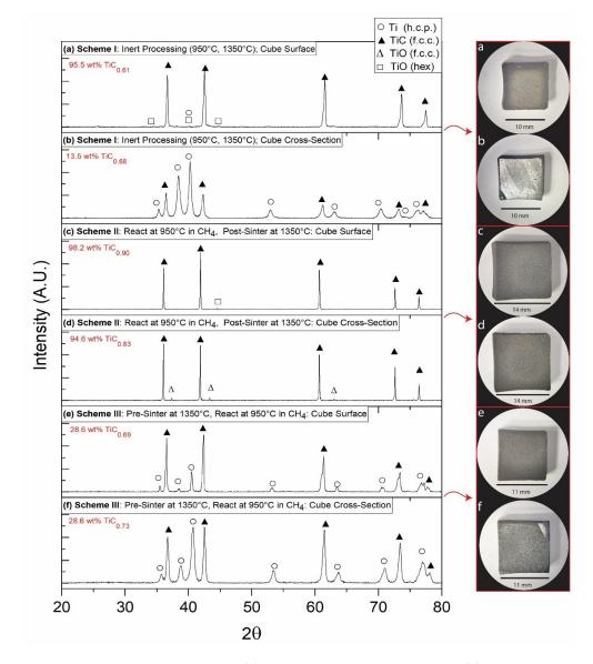
**Figure 8.** XRD spectra of post-processed Ti+phenolic parts converted to  $TiC_x$ . For each processing scheme, the optical images of the sample surfaces and cross-sections used for analysis are shown (a-f).
