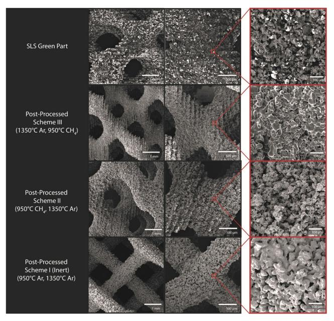
Figure 11. SEM images of lattice structures prior to post-processing (a) and after post-processing Schemes I-III (b-d). Samples are presented in order of descending macroscopic lattice size.
