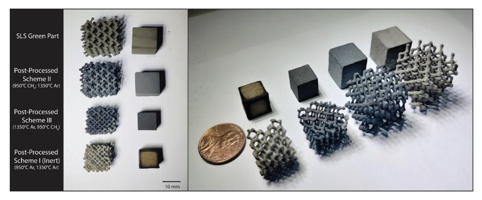
Figure 9. Photographs of the SLS green part in comparison to the post-processed samples converted to  $TiC_x$  containing structures using Schemes I-III.
