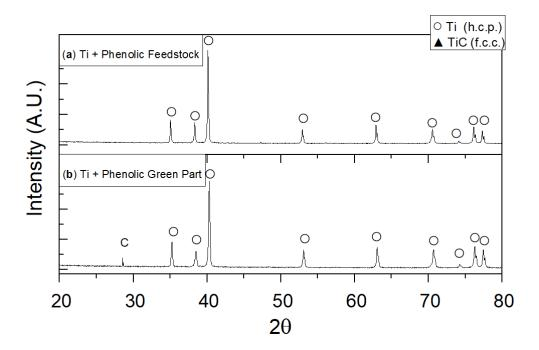
**Figure 7.** XRD spectra of unreacted 75 vol% Ti powder+ 25 vol% phenolic resin feedstock (a), green-state sample (b) after SLS processing to structures shown in Figure 6.
