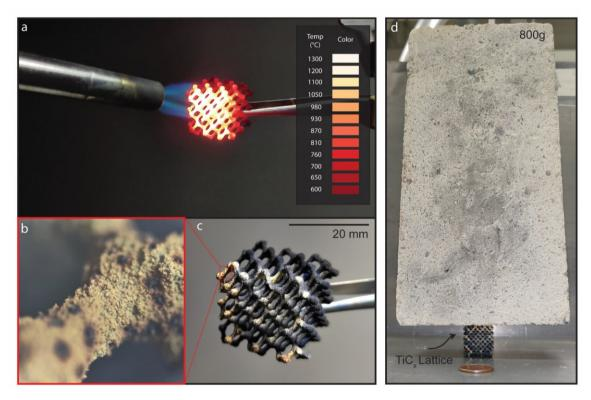
**Figure 14.** Photograph still from the recorded blow torch test (a) and optical micrograph of resulting microstructure (b), and photographs of the product lattice (c). (d) shows the lattice after heating supporting an 800 g alumina firebrick to illustrate its qualitative mechanical properties; a penny is shown for scale.
