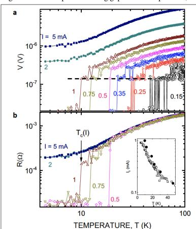
**Figure 3. Superconducting transition. a:**  $V = V_{9-10}(T, B = 0)$  measured at various currents  $I = I_{1-11}$  at B = 0 varying from  $I=5\mu$ A to  $I=0.15\mu$ A; the dashed line corresponds to the voltage level  $V = 0.15\mu$ V. **b:** R(T) = V(T)/I obtained from (**a**) for these selected currents; the inset presents  $I_c(T)$  (•) together with the data of Fig.2c ( $\Box$ ) for  $I_c(T,B=0)$ .
