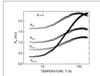
Figure 6. Temperature dependencies of the normal state resistance,  $R_{ik}(T) = V_{ik}(T)/I_{1-11}$ , obtained from the measurements in the local configuration, with current flowing between electrodes 1 and 11,  $I_{1-11} = 5$  mA, and voltages  $V_{ik}(T)$  measured in the current-applied region.
