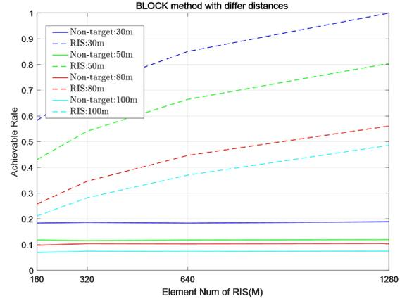
**FIGURE 15.** Performance of the RIS using blocking mechanism deployed at different distances from the NB
