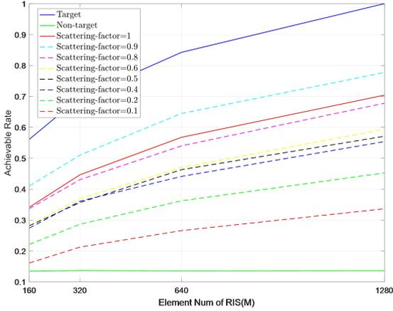
**FIGURE 9.** Nontarget signal performance of the RIS with a multiple-layer structure
