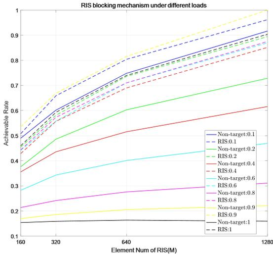
**FIGURE 14.** Performance of the RIS blocking mechanism under different loads
