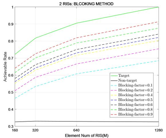
**FIGURE 16.** Performance achieved when two RISs using blocking mechanism are deployed in a cell
