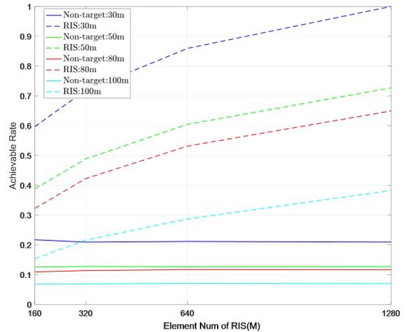
**FIGURE 11.** Performance of the RIS with a multilayer structure when deployed at different distances from the NB
