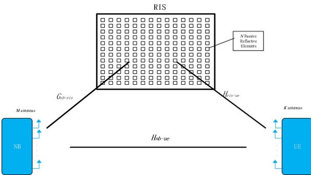
$H_{nb-ue} \in C^{K \times M}$  represent the direct channel between the user and the NB;  $G_{nb-ris} \in C^{N \times M}$  is the channel between the RIS and the NB, and  $H_{ris-ue} \in C^{K \times N}$  is the channel between the user and the RIS.
