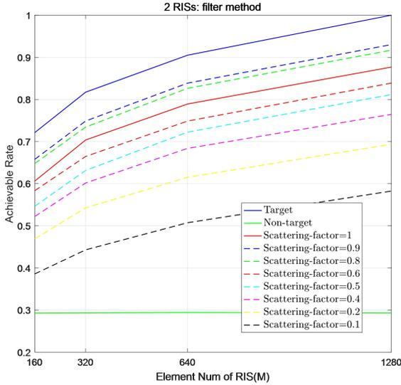
**FIGURE 12.** Performance of the RIS with a multiple-layer structure when two RISs are deployed in a cell
