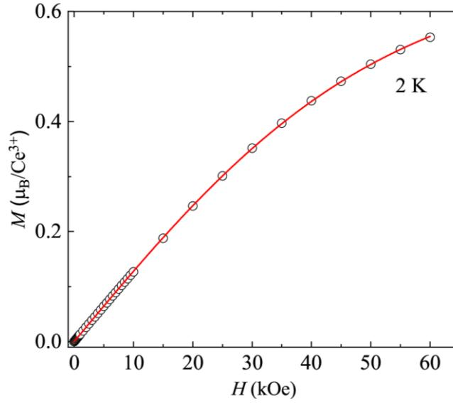
**Fig. 6:** Isothermal magnetization curve,  $M(H)$  at 2 K. The solid red line shows the simulation to the Brillouin function for  $J = \frac{1}{2}$ , with  $g_J \sim 1.13$ .
