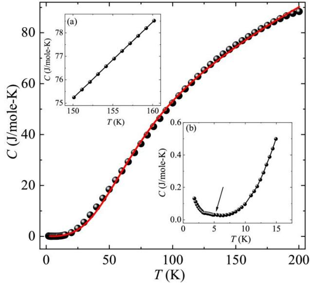
**Fig. 7:**  $T$  dependent heat capacity at 0 Oe up to 200 K with solid red line showing fit to the equation (2). Inset (a) shows the same data in the region where a step like behaviour is observed in  $\chi_{DC}$ . Inset (b) shows the expanded view of the same data below 15 K with the solid black arrow indicating the upturn.
