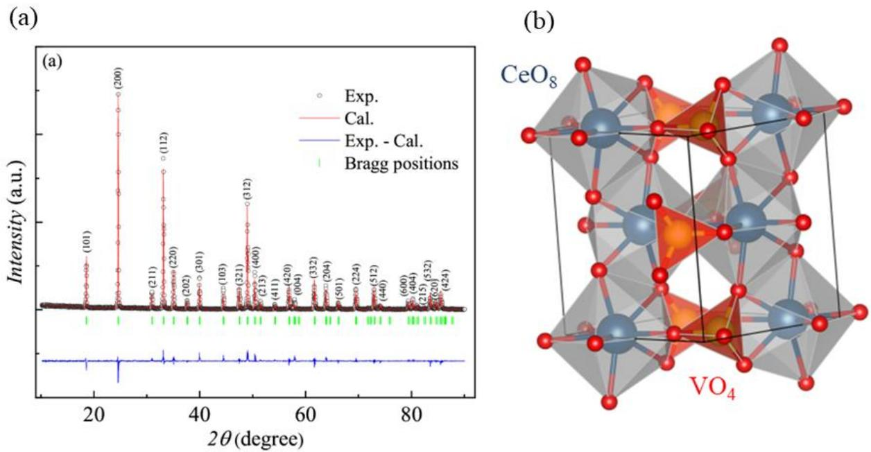
**Fig 1:** (a) Rietveld refined powder-XRD pattern of CeVO<sub>4</sub>. The black open circles indicate the experimental data, while the Rietveld refinement fit is shown as solid red line. The difference curve and the Bragg positions are shown by solid blue line and green vertical lines, respectively. (b) Crystal structure of CeVO<sub>4</sub>, comprised of CeO<sub>8</sub> polyhedral and VO<sub>4</sub> tetrahedra.
