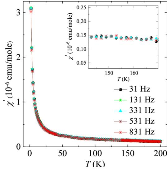
**Fig. 4:**  $T$  dependence of  $\chi'$  at various frequencies 31 – 831 Hz for zero applied DC field. Inset shows the expanded view of the same data.
