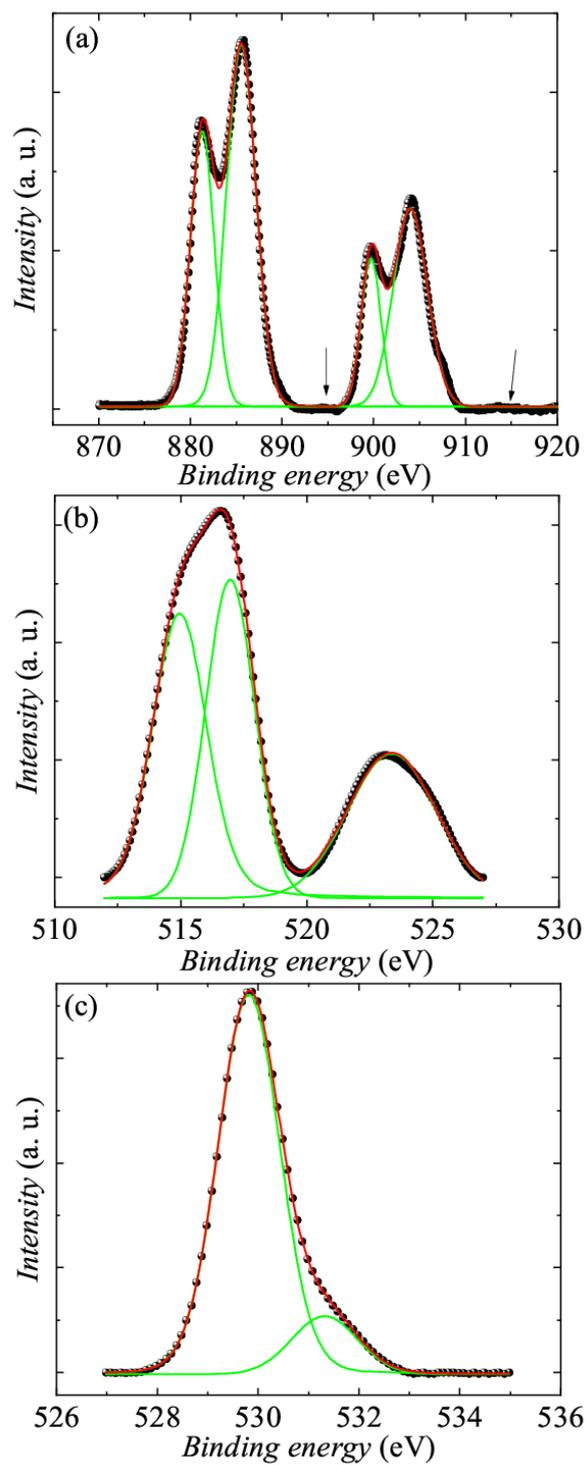
**Fig. 2:** (a, b, c) Room temperature X-ray photoemission spectra (XPS) of the core level of Ce 3d, V 2p, and O 1s, respectively. The solid red and green lines show the resultant fit and individual peak fittings, respectively.
