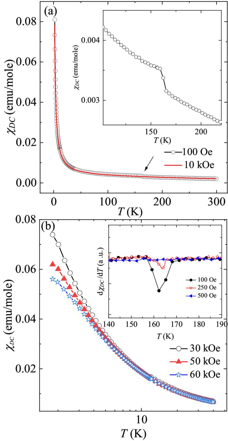
**Fig. 3:** (a)  $T$  dependent  $\chi_{DC}$  at 100 Oe and 10 kOe. The arrow indicates the inflection point observed in the 100 Oe curve. Inset: Same curve in the expanded region in the neighbourhood of inflection point. (b)  $\chi_{DC}$  vs  $T$  curves obtained at various applied fields on the log scale. Inset: Derivative of  $\chi_{DC}$  with respect to temperature at various fields up to 500 Oe measured under ZFC protocol.
