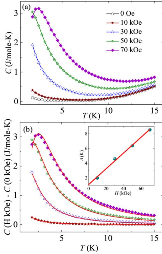
**Fig. 8:** (a)  $T$  response of heat capacity at various applied  $H$  up to 70 kOe. (b) Heat capacity after subtracting the zero-field data. The solid red lines show the fit to two-level Schottky scheme. Inset: Energy gap variation with the externally applied  $H$  along with the linear fitting (shown by the solid red line).
