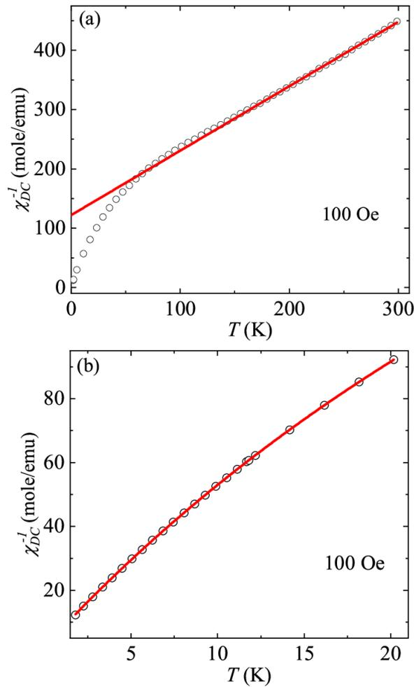
**Fig. 5:** (a)  $\chi_{DC}^{-1}$  as a function of  $T$  at 100 Oe. The solid red line shows the fitting to the CW law in higher temperature region. (b)  $T$  dependent  $\chi_{DC}^{-1}$  at 100 Oe below 20 K, with solid red line showing the fit to the modified CW law.
