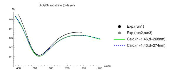
FIG. 9. **Determination of SiO**<sub>2</sub> thickness. Measured (black [run 1] and gray [run 2 (run 3)] dots) and calculated (green and blue dashed curves) spectral reflectivities of N-layer graphene on the same SiO<sub>2</sub>/Si substrate. A white-light source was used, and the reflectivity was measured at room temperature. The horizontal axis is  $\lambda$  (nm), and the reliable range of our spectrometer is 450 to 800 nm.
