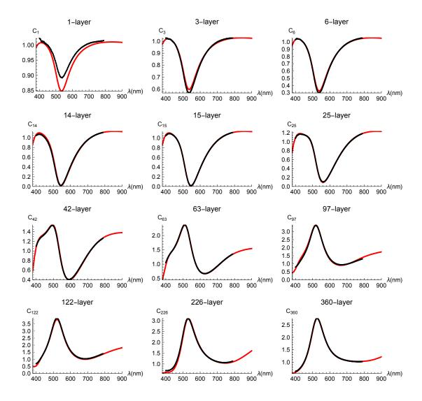
FIG. 1. Measured (black circles) and calculated (red solid) spectral contrasts of N-layer graphene on the same SiO<sub>2</sub>/Si substrate. The measurments were conducted using a white-light source at room temperature. The red solid curves were obtained from Eq. (1) with  $\varepsilon_g = (n+ik)^2$  using optical constants obtained by El-Sayed *et al.* [19] The horizontal axis is  $\lambda$  (nm), and the reliable range of our spectrometer is 450 to 800 nm.
