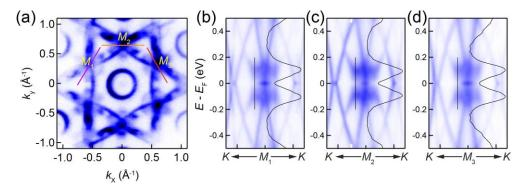
Figure S7: (a) Constant energy counters of ARPES mapping taken at Fermi surface. (b-d) Band dispersion cut along K - M - K direction at three different M point ( $M_{1,2,3}$  marked in (a)). The data were symmetrized with respect to  $E_F$ . The energy distribution curves across the dark straight line are appended in corresponding sub-figures.
