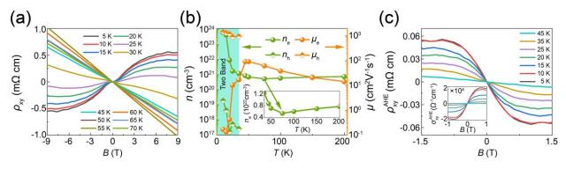
Figure S19: (a) Hall resistivity of  $KV_3Sb_5$  with in-plane current and out-of-plane magnetic field. (b) Temperature dependent measurement of electron carrier concentration and mobility of  $KV_3Sb_5$  (The data was fitted with two band model below 50 K). Inset: the enlarged curves around CDW transition temperature. (c) Extracted  $\rho_{xy}^{AHE}$  and  $\sigma_{xy}^{AHE}$  (inset) at various temperature.
