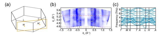
Figure S10: (a) *MLL'LM* plane (yellow frame) of the BZ going through the nesting region. (b) Experimental out-of-plane FS cuts in the *MLL'LM* plane. 3D warping of the FS counter is indicated by dashed yellow curves and Brillouin zone boundaries are indicated by red dashed lines. (c) The DFT calculated phonon spectrum of KV<sub>3</sub>Sb<sub>5</sub>.
