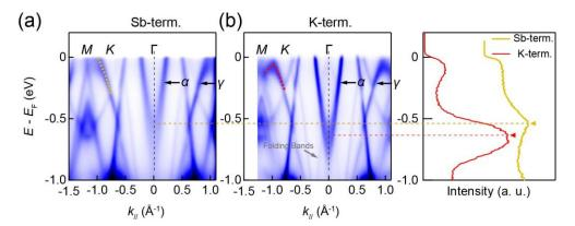
Figure S5: (a) Band dispersion cut along— $M K \Gamma$ –K M direction on domain without folding bands; (b) Band dispersion cut along–M- $K \Gamma$ –K M direction on domain with folding bands; (c-e) Energy distribution curves cut along dark dash line illustrated in (a) and (b), the gold curve is extracted from (a) and red curve is extracted from (b).
