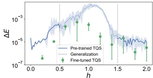
FIG. 4. Relative error of the ground state energy of the TFI Hamiltonian, Eq. (7), with  $n = 40$ . Lines and data points are medians of 10 estimations, while shaded regions and error bars enclose 10<sup>th</sup> to 90<sup>th</sup> percentile. Dotted lines are generalizations to regions TQS has not been trained on. Data points below  $10^{-7}$  are not shown for a clearer illustration.
