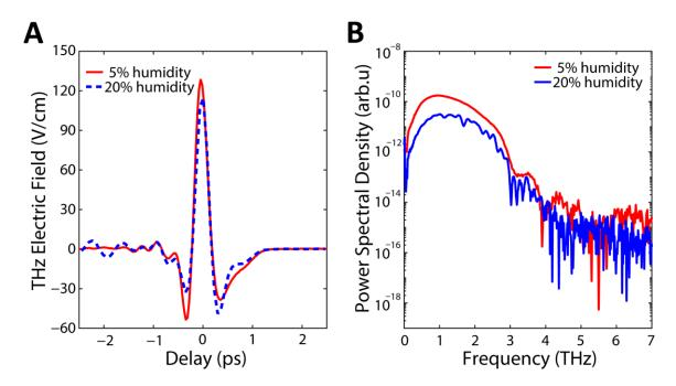
**Figure 1.** (A) THz time-domain spectroscopy using electro-optic sampling to characterize the THz field trace and spectrum using a classical balanced detection scheme. (B) Power spectrum corresponding to the measurement in (A). The blue curves are for an un-purged setup (blue curve) while the red curves show the result in a pure nitrogen atmosphere.
