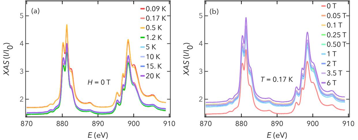
Fig. S4: (a & b) Raw Ce-XAS for CeCoIn<sub>5</sub> at M<sub>5,4</sub> absorption edges of cerium as a function of external magnetic field and temperature.
