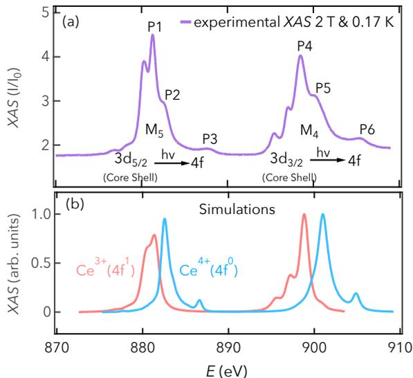
FIG. 2. (a) Ce-XAS normalized by the incoming light intensity ( $I_0$ ) acquired at 0.17 K under an applied external magnetic field of 2 T. The spectrum clearly shows observation of  $M_{5,4}$  resonance edges of Ce along with various satellite features (P2, P3, P5, and P6). (b) Simulated XAS for  $Ce^{3+}/Ce^{4+}$  using the CTM4XAS software [27].
