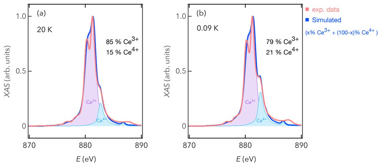
Fig. S3: (a) Ce-XAS for CeCoIn<sub>5</sub> at M<sub>5</sub> absorption edge at 20 K with simulated data shown in the same graph. Simulated curve at 20 K has 85% Ce<sup>3+</sup> and 15% Ce<sup>4+</sup> contribution which is the best estimate for the given simulations. (b) Ce-XAS for CeCoIn<sub>5</sub> at M<sub>5</sub> absorption edge at 0.09 K with simulated data. Simulated curve at 0.09 K shows an increased contribution of 21% Ce<sup>4+</sup> from 15% at 20 K.
