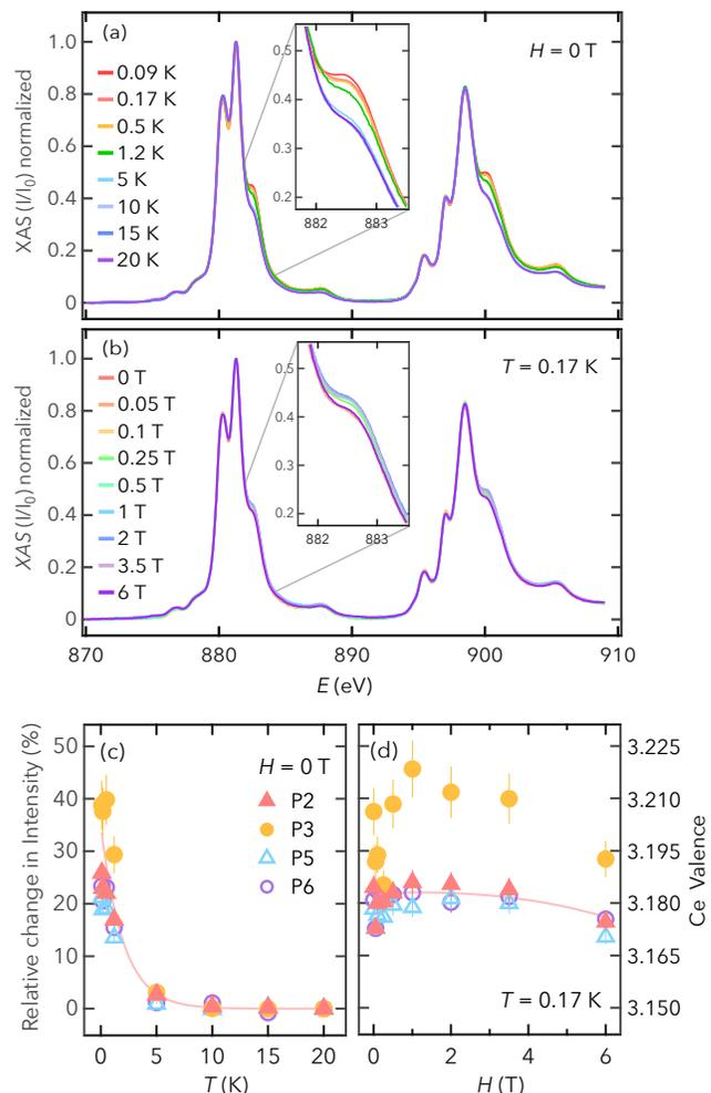
FIG. 3. (a) Isotropic Ce- $M_{5,4}$  XAS of  $CeCoIn_5$  as a function of temperature (normalized with respect to P1). (b) XAS as a function of applied external magnetic field. (c) Relative intensity change of the  $Ce^{4+}$  absorption multiplets (Ce valence on right axis) as a function of temperature with the 20 K curve as reference. (d) Corresponding change as a function of magnetic field, using the same 20 K reference. Curves connecting data points in (c) & (d) are guide to the eye.
