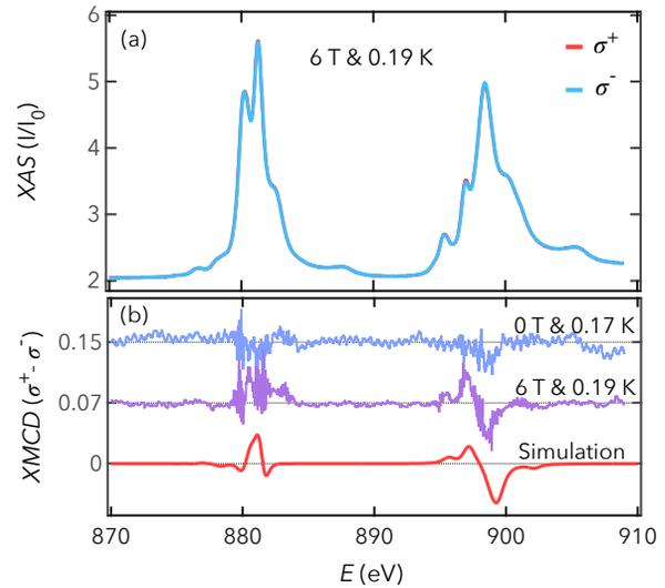
FIG. 4. (a) Ce-XAS obtained by parallel ( $\sigma^+$ ) and antiparallel ( $\sigma^-$ ) circular polarized x-ray at 0.17 K and 6 T. (b) Simulated and experimental XMCD (0.17 K & 0.19 K) for Ce at fields 0 & 6 T. XMCD is the difference of  $\sigma^+$  and  $\sigma^-$  XAS and matches with the simulated curve for experimental 6 T. Baseline are shifted for visualization and are 0.150 and 0.075 for 0 & 6 T curve, respectively.
