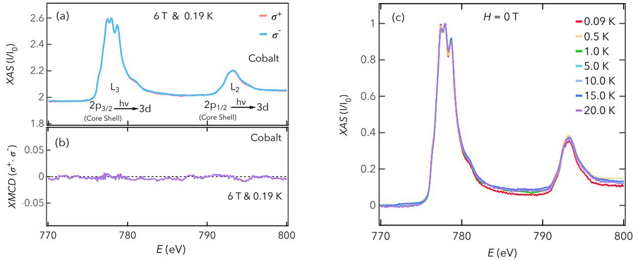
Fig. S5: (a) Co-XAS obtained by parallel ( $\sigma^+$ ) and antiparallel ( $\sigma^-$ ) circular polarized x-ray at 0.19 K and 6 T. (b) Co-XMCD at 0.19 K and 6 T. (c) Temperature dependence of normalized isotropic XAS of Co at zero external magnetic field.
