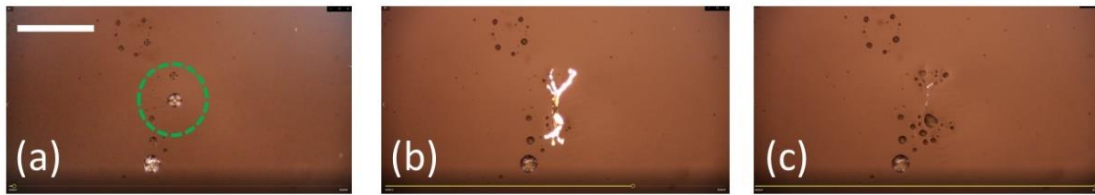
Fig. 9. A small E7 droplet on the X-cut LN-Fe plate positioned in the middle of the illuminated area during laser irradiation at room temperature. (a) At the starting of laser illumination, (b) 28 s afterward, (c) 41 s afterward. The location of a laser beam is indicated by the green circle in (a). The scale bar is 1 mm. (Full video is available in the supplementary material (video S10)).
