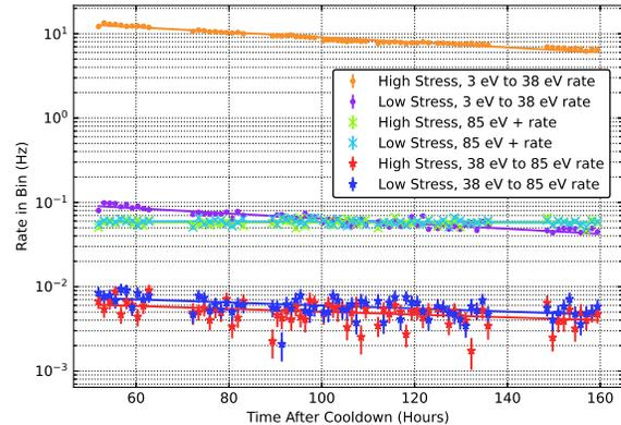
FIG. 3. **Time dependence of background rates in High Stress (light colors) and Low Stress (dark colors) calorimeters.** Rates are measured in three energy bins: 3–38 eV, 38–85 eV, and 85+ eV. Exponential fits are shown as solid lines.
