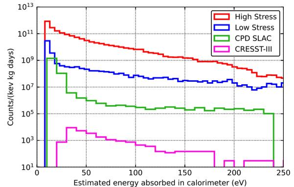
FIG. 4. **Comparison to CPD and CRESST.** Spectra of events in HS and LS calorimeters, compared to those measured with the CRESST-III detector [17] and by SuperCDMS in the CPD detector at SLAC [16]. Data are from the last of seven datasets taken. The energy in the HS and LS calorimeters are estimated assuming a phonon collection efficiency of 12.5%, and therefore differ by a constant factor from the spectra in Fig. 2.
