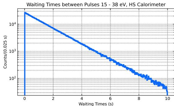
FIG. 6. **Waiting Time Distribution in the High Stress Calorimeter.** Time until another event (“waiting time”) in the 15–38 eV energy range in a high stress calorimeter. We expect events in this energy range to be primarily composed of microfracture events. The data are well-described by a Poissonian model, in contrast to those in Ref. [25].
