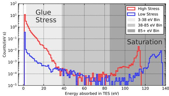
FIG. 2. **Background spectra of energy absorbed in TESs in High Stress and Low Stress calorimeters.** The histogram is divided into three regions: high energies associated with saturation (85+ eV), and two lower-energy bins (38–85 eV; 3–35 eV) where the backgrounds appear to be similar and different in the two calorimeters, respectively. These spectra are from a 12 hour dataset, the last of 7 datasets acquired (see Appendix E).
