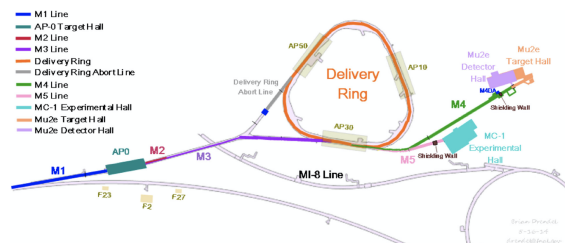
FIG. 1: A schematic representation of the Muon Campus at Fermilab.
