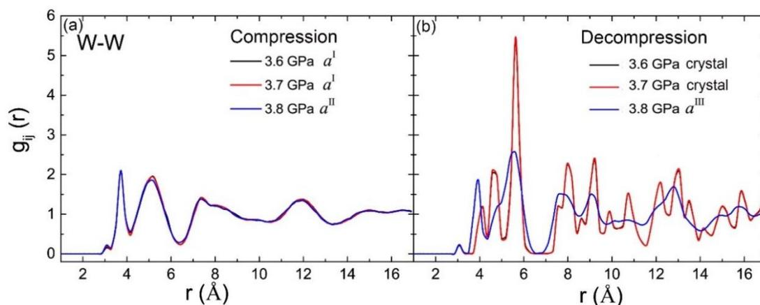
**Fig. 8 Partial W-W RDFs of  $ZrW_2O_8$  at different pressures.** (a) RDFs at different pressure, (b) RDFs upon decompression.
