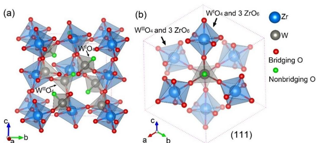
**Fig.1 Structure of cubic  $\text{ZrW}_2\text{O}_8$  unit cell.** (a) The cubic cell consists of a network of corner-shared octahedral  $\text{ZrO}_6$  and tetrahedral  $\text{WO}_4$ . The octahedral  $\text{ZrO}_6$  are equivalent but the
