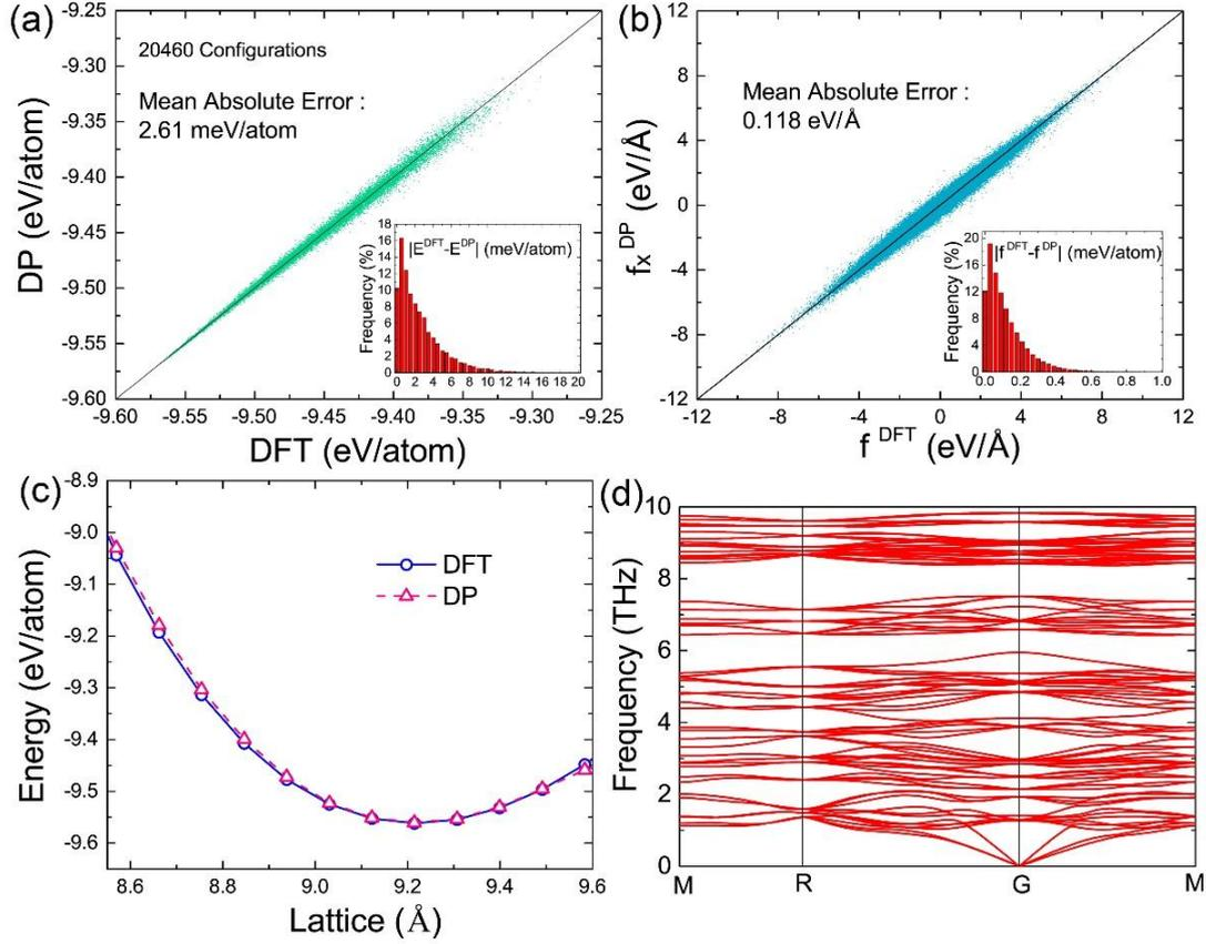
**Fig. 2 The benchmark test of DP against DFT results.** Comparison of energies (a) and atomic forces (b) calculated using the DP and DFT for all configurations. DP and DFT energies for different hydrostatic pressure (c) and phonon dispersion relations (d) for cubic phase.
