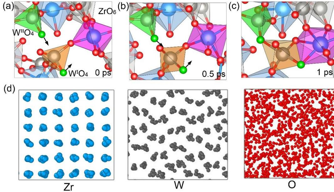
**Fig. 7 Atomic structure evolution of amorphous  $ZrW_2O_8$  at 3 GPa.** (a)-(c) the movement of nonbridging O (marked in green) result in formation of  $ZrO_7$  decanedron and  $WO_5$  octahedron. (d) A part snapshot of amorphous 22528-atom supercell, the arrangements of Zr, W, and O are presented respectively.
