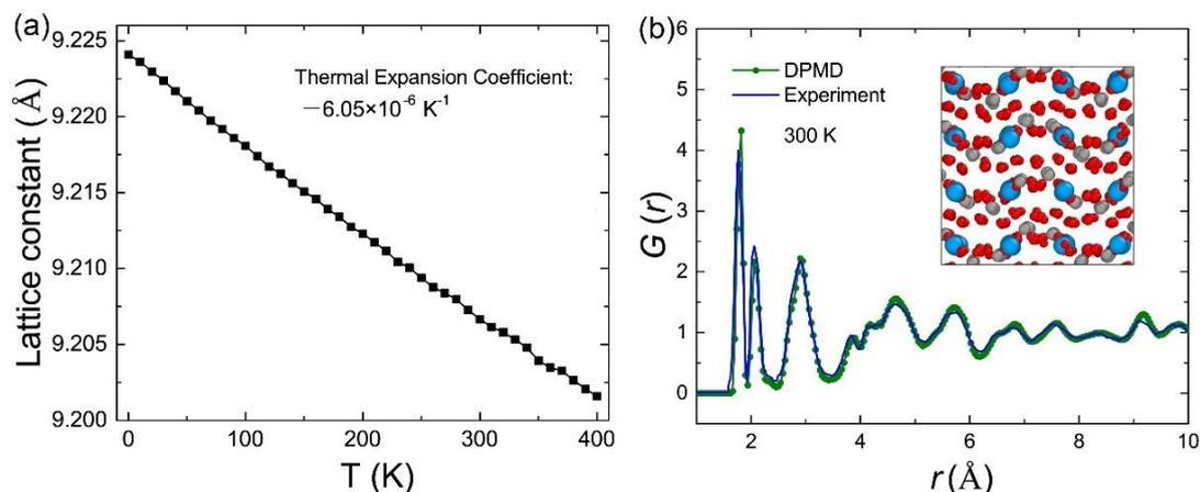
**Fig. 3 Crystal structural properties of  $\text{ZrW}_2\text{O}_8$  on heating.** (a) Variation of cubic  $\text{ZrW}_2\text{O}_8$  lattice parameter with temperature from DPMD at ambient pressure. (b) Neutron weighted pair distribution functions  $G(r)$  from cubic  $\text{ZrW}_2\text{O}_8$  at 300 K and 1 bar calculated from DPMD and experiment.
