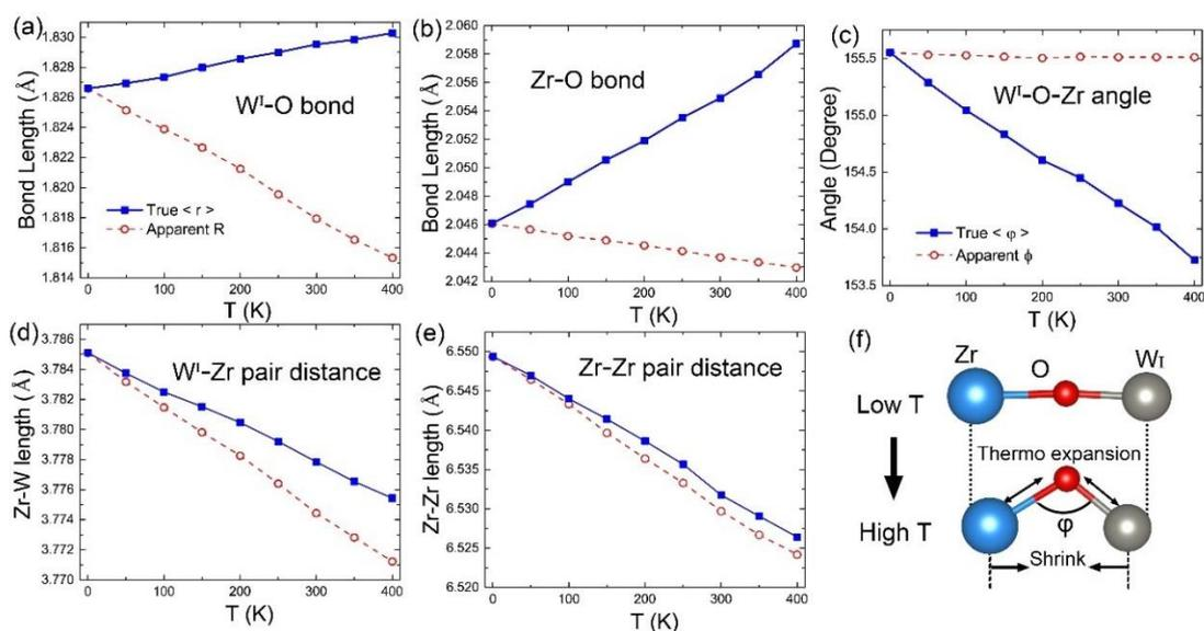
**Fig. 4 Thermal expansion of neighboring atom pair distances and degree of corner-sharing polyhedrons.** “True” and “apparent” bond length/atom pair of (a) W-O, (b) Zr-O, (d) Zr-W, (e) Zr-Zr, and angle of (c) Zr-O-W as a function of temperature. (f) The sketch of bond length and angle variation on heating.
