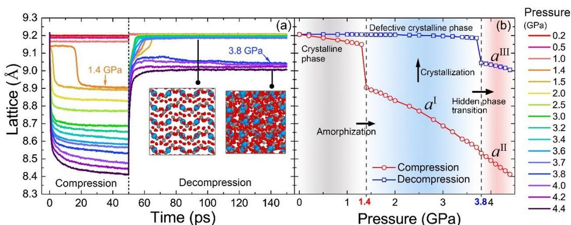
**Fig. 5 Structural properties of  $\text{ZrW}_2\text{O}_8$  with compression and decompression.** (a) Variation of lattice parameter with time on compression from 0.2 GPa to 4.4 GPa at 300 K and then upon decompression. (b) The lattice parameter depends on pressure for compression after 50 ps (red line) and decompression after 100 ps (blue line).
