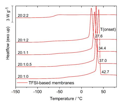
Figure S2: DSC cooling curves (after the shown heat ramp) of TFSAM-based ternary electrolytes with different PEO:salt:IL ratios; onset point of the crystallization peaks are marked (analysed with Universal Analysis 2000 from TA Instruments).
