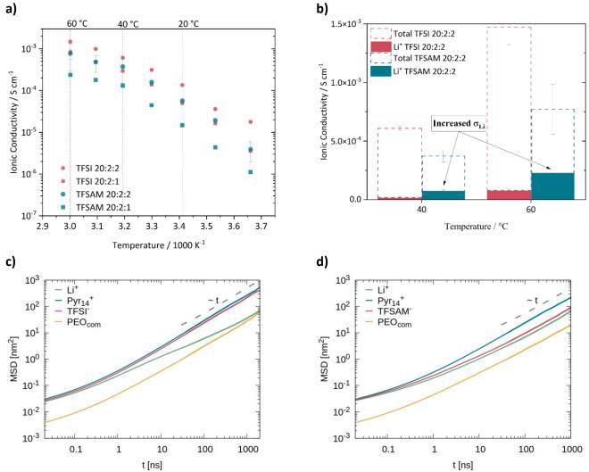
Figure 5: **Top row: a)** Temperature dependent ionic conductivities of TFSAM and TFSI based ternary electrolytes with PEO:salt:IL ratios 20:2:1 and 20:2:2; **b)** total ionic conductivity and portion of the conductivity contributed by Li<sup>+</sup> at 40 and 60 °C; **bottom row**: mean squared displacements of all molecular constituents in **c)** the TFSI-based and **d)** the TFSAM-based mixture.
