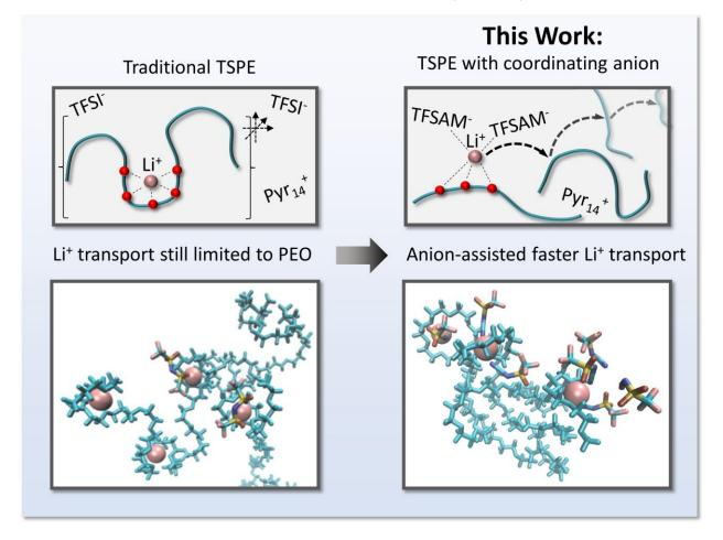
Figure 6: Novel, faster 'anion-assisted' transport mechanism (TFSAM-based) compared to the traditional Li<sup>+</sup> transport in TFSIbased TSPEs.
