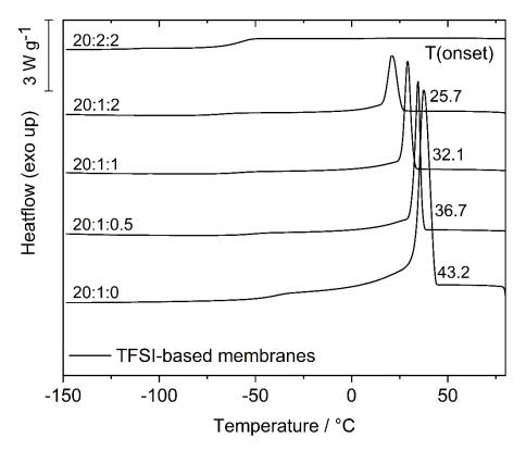
Figure S1: DSC cooling curves (after the shown heat ramp) of TFSI-based ternary electrolytes with different PEO:salt:IL ratios; onset point of the crystallization peaks are marked (analysed with Universal Analysis 2000 from TA Instruments).
