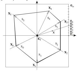
FIGURE 6. Polar slabs decomposition of a convex polygon
