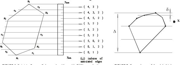
**FIGURE 4.** Point-in-Convex Polygon algorithm with O(1) complexity **FIGURE 5.** Dependence of the slab thickness However, the thickness of all slabs is not infinitely small. The thickness of all slabs is determined by geometric properties of the given convex polygon, actually by the smallest distance in the *y* coordinates, see Fig.5.
