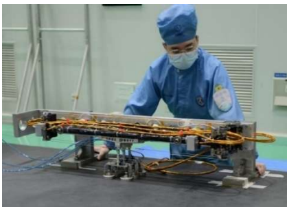
Fig. 13: MAG deployment test: Left – At instrument level, CAS/NSSC. Right – At ESA's European Space Research and Technology Centre (ESTEC), The Netherlands, after integration with the PLM.
