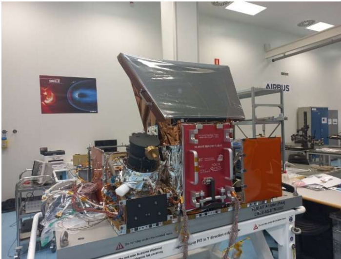
Fig. 11: STM SXI (large structure in the centre) and UVI (black cylinder on the left) mounted on the STM PLM, before shipping to China from Spain. Credit: Airbus, Madrid, Spain.
