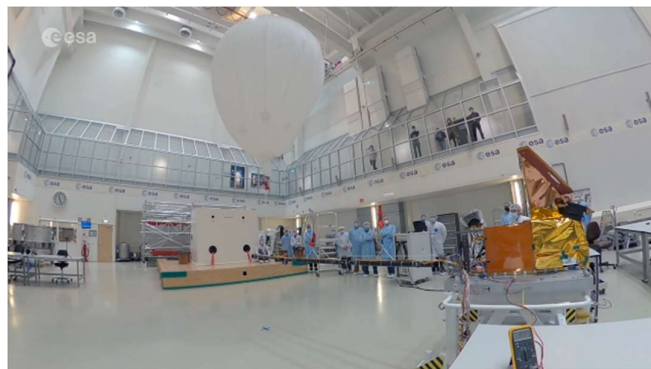
Fig. 13: MAG deployment test: Left – At instrument level, CAS/NSSC. Right – At ESA's European Space Research and Technology Centre (ESTEC), The Netherlands, after integration with the PLM.
