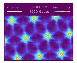
FIGURE 1. Experimental picture of the Abrikosov lattice obtained using a tunnelling microscope. Different colours signify different densities of super-conducting electrons. Theoretical description of this experiment is given solving the BdG system based on the coarse-scale approximation given by the Ginzburg-Landau system.
