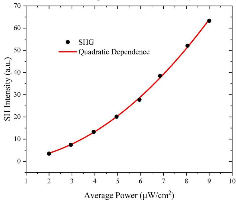
Fig S1. Power-dependent SHG response of TaAs (112). The dot and line correspond to data points and quadratic fitting.
