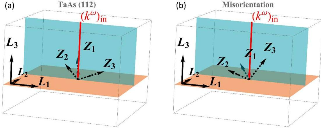
Fig S2. Relation between crystal physics axes ( $Z_1, Z_2, Z_3$ ) and lab coordinates ( $L_1, L_2, L_3$ ). Blue and orange planes are the plane of incidence and surface plane, respectively. **a** TaAs(112) with  $[1 -1 0]$  parallel to  $L_2$ . **b** Misorientation with  $[1 1 -1]$ ,  $[1 -1 0]$  and  $[1 1 2]$  parallel to  $L_1, L_2$  and  $L_3$ .  $(k^{\omega})_{in}$  is the incident wave vector.
