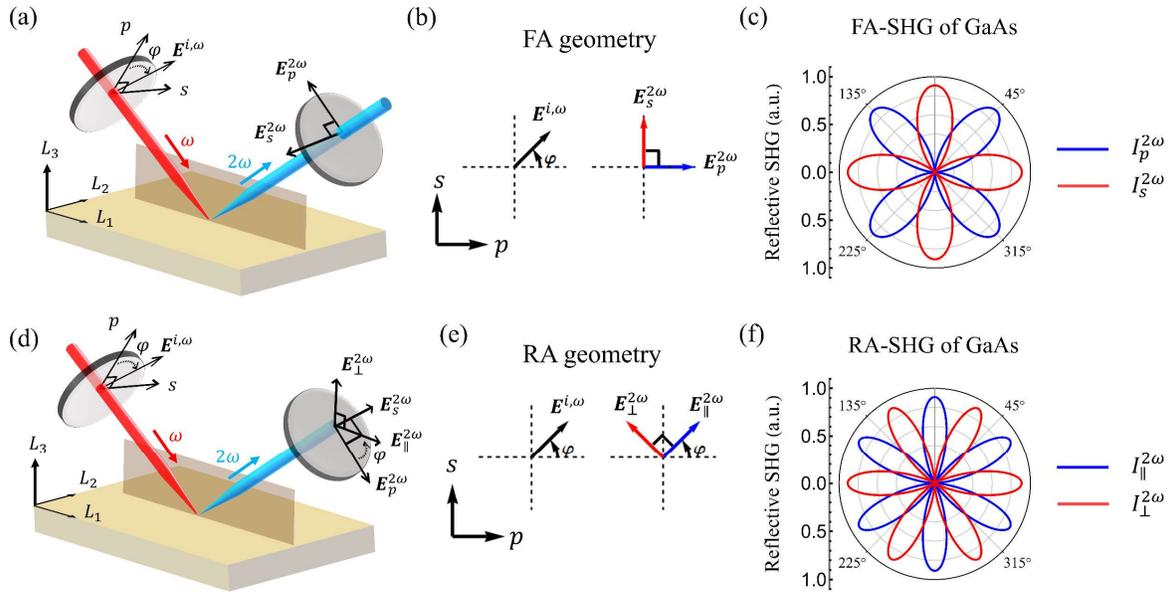
Figure 1. Two common experimental geometries for SHG polarimetry and the resulting reflection SHG polarimetry for GaAs(111) surface in normal incidence. **a-c** Rotating polarizer fixed analyzer (FA) geometry: SHG intensities of  $p$ - and  $s$ - polarized waves are recorded as a function of the azimuthal angle  $\varphi$ . **d-f** Rotating polarizer, rotating analyzer (RA) geometry: SHG intensities polarized parallel or perpendicular to the incident polarization are recorded as a
