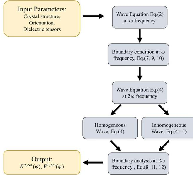
Figure 3. Flowchart illustrating the key steps in deriving the polarized second harmonic fields generated by a nonlinear medium.
