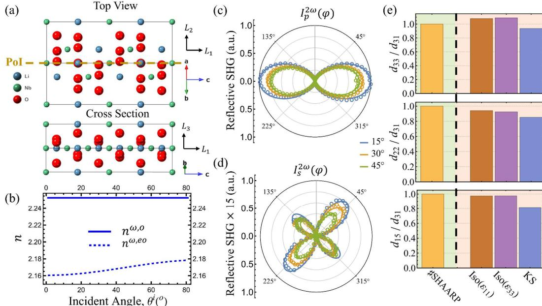
Figure 5. Linear and nonlinear optical response of LiNbO<sub>3</sub> (11 $\bar{2}$ 0). **a** Crystal structure and experimental orientation. **b** The real part of the effective refractive indices at  $\omega$  frequency as a function of incident angle ( $\theta^i$ ). **c-d**  $p$ - and  $s$ -polarized second harmonic response as a function of azimuthal angle ( $\varphi$ ) at various incident angles ( $\theta^i$ ). **e** Comparison
