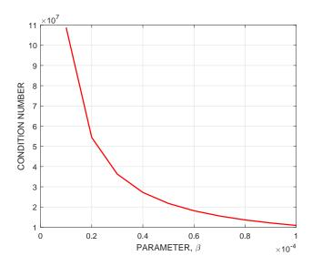
Figure 2: The condition number of the matrix  $A_{rk}$  in (40) as a function of the regularization parameter  $\beta > 0$  is plotted. For a small  $\beta$  the matrix  $A_{rk}$  is ill-conditioned matrix for which the spectral radius  $\rho(I - S_k^{-1}A_{rk})$ , where  $S_k^{-1} = I/\alpha_k$  with  $\alpha_k = ||A_{rk}||_{\infty}/2 + \varepsilon$  is very close to one.
