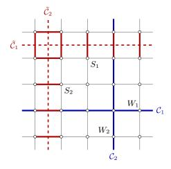
FIG. 8. Graphical representation of the non-local order parameters  $\overline{W}_{1,2}$  (in blue) and  $\overline{S}_{1,2}$  (in red) and their respective paths  $C_{1,2}$  and  $\tilde{C}_{1,2}$ .
