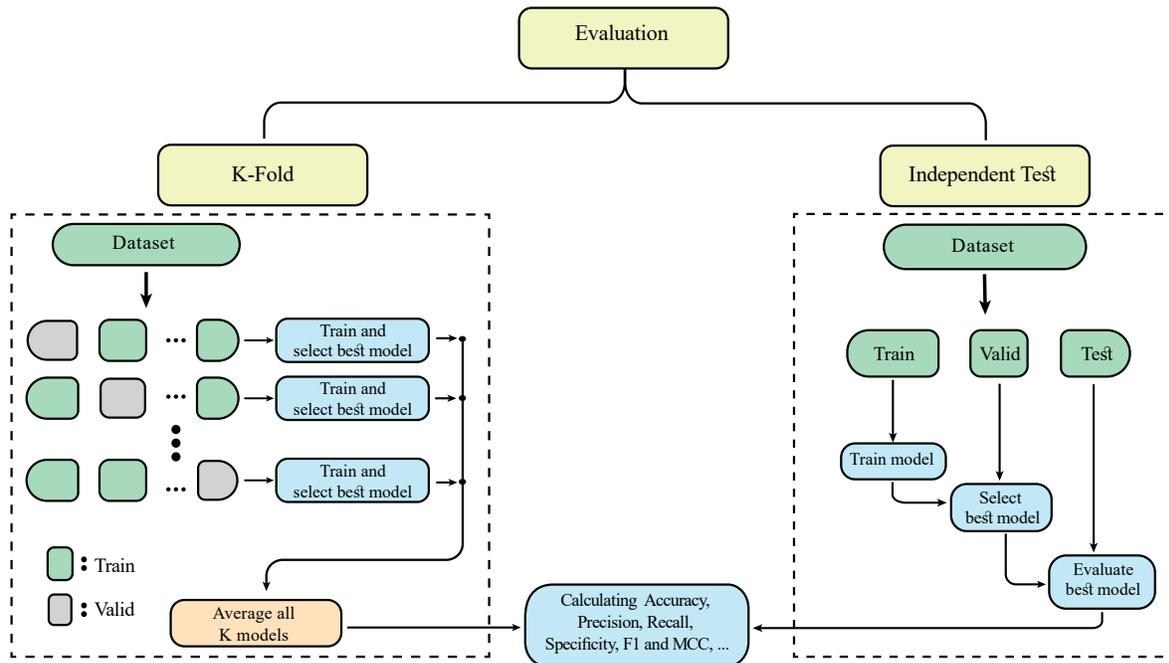
**Figure 6:** The evaluation step can be done by two methods: K-fold cross validation and independent test. Independent test method sometimes is called “Train-Test” or “Train-Valid-Test” as well.
