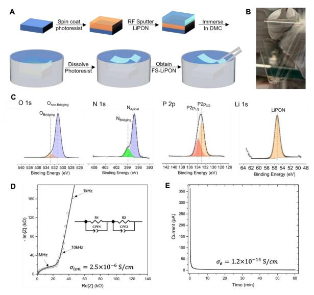
**Figure 1.** (A) Schematic of synthesis procedure for FS-LiPON. (B) Optical photo of a transparent and flexible FS-LiPON thin film. (C) XPS spectra of O 1s, N 1s, P 2p and Li 1s regions of FS-LiPON thin film. (D) EIS plot and (E) DC polarization plot of FS-LiPON.
