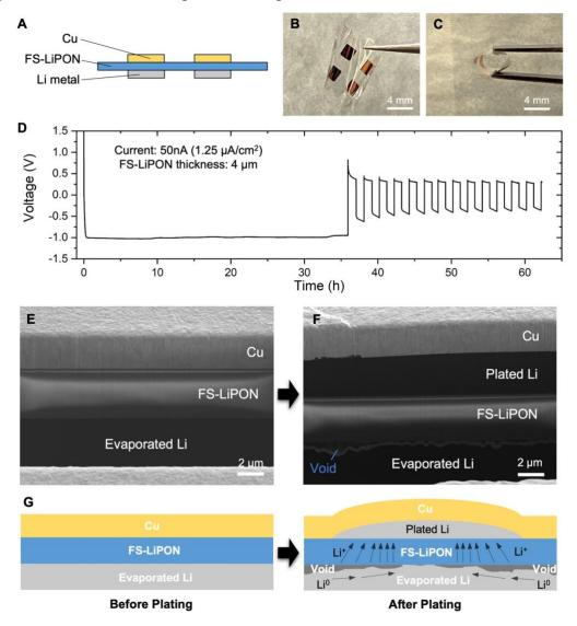
**Figure 3.** (A) Cross-section schematic of the FS-LiPON Li-Cu cell. Photos of FS-LiPON Li-Cu cell from top view (B) and upon bending (C). (D) Voltage curve of Li metal plating and stripping in a FS-LiPON Li-Cu cell. Cross-section cryo-FIB/SEM images of Li-Cu cell before Li metal plating (E) and after Li metal plating (F). The plated capacity in (F) is ~0.31 mAh/cm<sup>2</sup>. (G) Schematic showing the proposed non-uniform void formation mechanism during Li metal plating.
