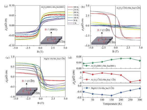
Figure 4 Hall resistivity measured as a function of out of plane applied magnetic field
