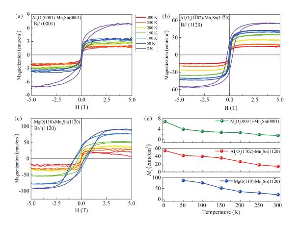
Figure 3 Temperature dependent magnetic hysteresis of Mn<sub>3</sub>Sn films (a) M-H curves measured between 2–300 K for the Al<sub>2</sub>O<sub>3</sub>/Mn<sub>3</sub>Sn (0001) film. (b) M-H curves measured at 2–300 K for the Al<sub>2</sub>O<sub>3</sub>/Mn<sub>3</sub>Sn (11 $\overline{2}$ 0) film. (c) M-H curves measured at 50–300 K for the MgO/Mn<sub>3</sub>Sn (11 $\overline{2}$ 0) film. (d) M<sub>s</sub>-T curves as a function of temperature for the three Mn<sub>3</sub>Sn films.
