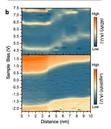
**Figure 4. (a)** STM image of a partially Se intercalated MoSe<sub>2</sub> island, sample bias V = -2 V, setpoint I = 10 pA. **(b)** 2D color rendering of  $(\partial Z/\partial V)_I$  (top) and dI/dV (bottom) spectroscopy obtained along the black line in the STM image.
