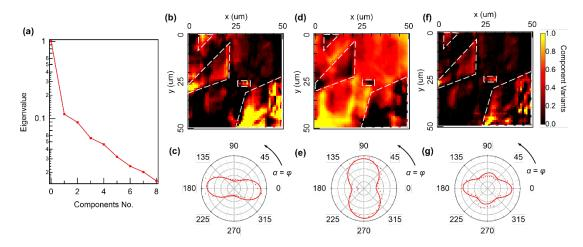
**Fig. 4.** Matrix decomposition analysis of SHG spectral imaging data. (a) Scree plot of variance ratio as a function of components number in the principle component analysis. (b,d,f) Component maps extracted from the original spectral imaging data by the three-component Bayes linear unmixing analysis and (c,e,g) corresponding SHG anisotropy spectra.
