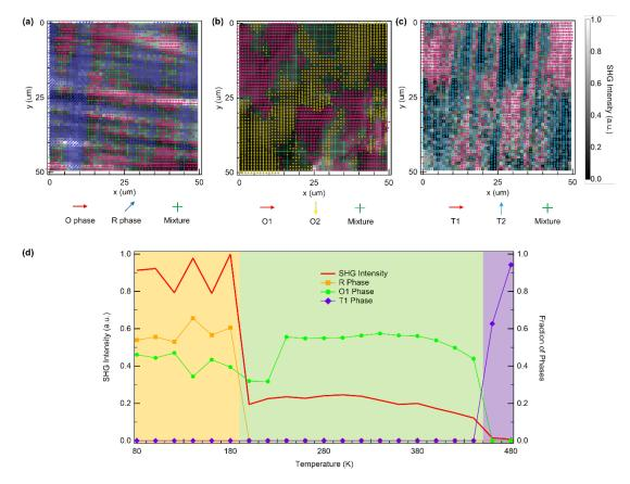
**Fig. 3.** Thermal evolution of domain configurations of KNN revealed by SHG spectral imaging. (ac) Analyzed 2D maps of phase and domain variants for the same region measured at 100 K, 280 K and 500 K, respectively. The color and direction of arrows denote the major domain type for each pixel. The overlaid SHG images were measured at  $\alpha = \varphi = 0^{\circ}$ . (d) Temperature-dependent domain fractions and corresponding SHG intensity summer over the measured region.
