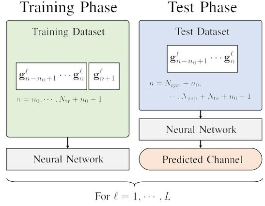
Fig. 1: Two-phase block diagram of the SL approach.
