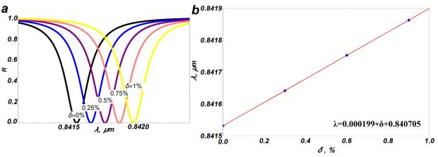
Fig. 7. (a) R spectra with changes in concentration; (b) Dependence of the DM peak on concentration; h<sub>d</sub>=0.325 μm. All other parameters are as in Fig. 3
