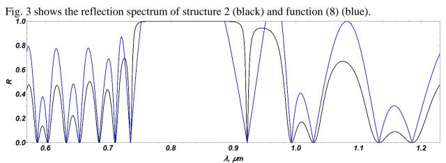
Fig. 3. Spectra of reflection (black) and function (8) (blue) for the structure 2. Parameters of structure  $h_1=0.14 \mu m$ ,  $h_2=0.10 \mu m$ ,  $h_d=0.44 \mu m$ ; N=10.
