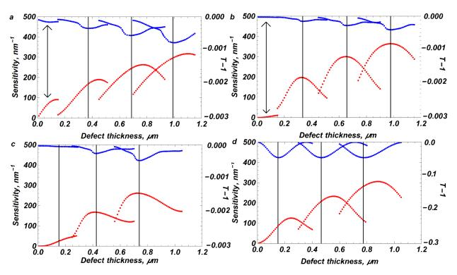
Fig. 6. Sensitivity and amplitude of the biosensor as a function of DL thickness, for 4 structure types: (a) structure 1, (b) structure 2, (c) structure 3, (d) structure 4. Blue points represent DM amplitudes, red points represent sensitivity (9), black lines represent the center of the PBG. The parameters are as in Fig. 2.
