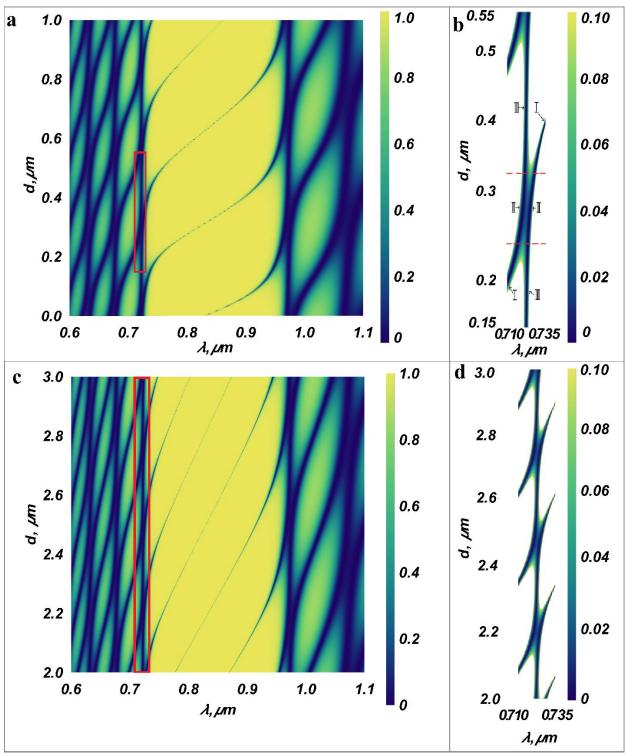
Fig. 4. (a,c) Dependence of reflection spectrum on the DL thickness for the structure 2; (b,d) zoomed in spectrum. All other parameters are as in Fig. 3.
