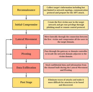
Fig. 1: APT attack stages. Yellow Blocks: initial and final stages. Red Blocks: attack stages.
