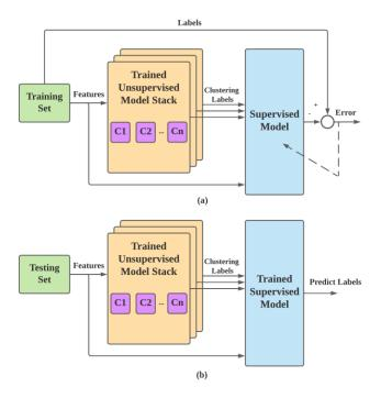
Fig. 2: (a) The training phase of the PKI model, (b) The testing phase of the PKI model
