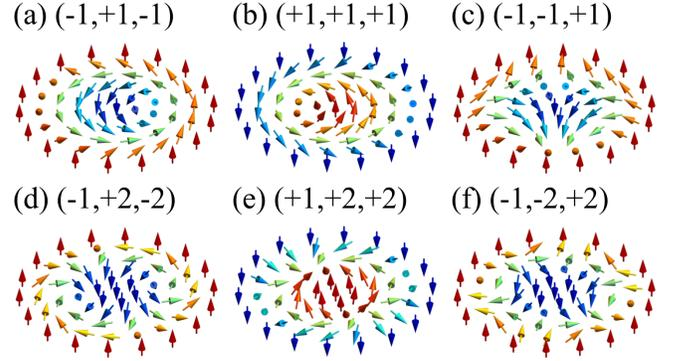
FIG. 1. Skyrmions characterized by  $(p, v, N_{\text{sk}})$ . The arrow and color show the spin direction and  $z$  component, respectively, where red (blue) corresponds to the positive (negative)  $z$  component.
