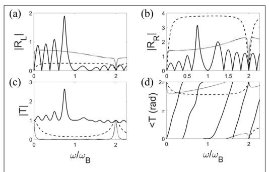
FIG. 4. Frequency response of the (a) magnitude of  $R_L$ , (b) magnitude of  $R_R$ , (c) magnitude of T, and (d) phase of T for the finite structure in Fig. 2(a) for  $\sigma_S$ =0.5 $\sigma_{TH}$  (solid lines),  $\sigma_S$ = $\sigma_{TH}$  (dashed lines), and  $\sigma_S$ =2 $\sigma_{TH}$  (dotted lines), where the threshold value  $\sigma_{TH}$  is equal to 3.4Y<sub>0</sub>.
