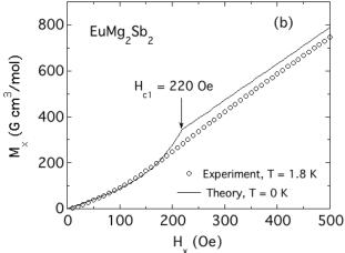
FIG. 9. Experimental magnetization  $M_x=M_{ab}$  versus magnetic field  $H_x=H_{ab}$  at T=1.8 K (open circles) and the theoretical predictions for T=0 K (solid curve) for (a) EuMg<sub>2</sub>Bi<sub>2</sub> with  $H_{c1}\approx 465$  Oe and (b) EuMg<sub>2</sub>Bi<sub>2</sub> with  $H_{c1}\approx 220$  Oe.
