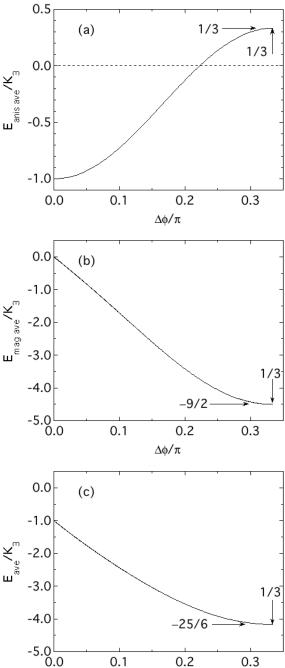
FIG. 4. (a) Average anisotropy energy  $E_{\rm anis\,ave}$ , (b) average magnetic energy  $E_{\rm mag\,ave}$ , and (c) the average total energy  $E_{\rm ave}$ , all normalized by the anisotropy constant  $K_3$ , versus the tilt angle  $\Delta\phi/\pi$  of the AFM moments in Fig. 3(a) except for the moments in Domain A for which  $\Delta\phi=0$ . The value  $|\Delta\phi|/\pi=1/3$  occurs at  $H_x=H_{\rm c1}$ .
