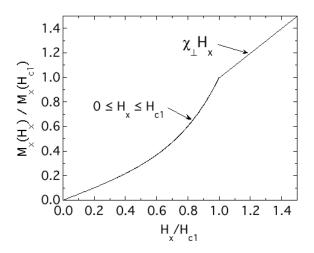
FIG. 7. Theoretical magnetization ratio  $M_x(H_x)/M_x(H_{c1})$  vs the field ratio  $H_x/H_{c1}$ . Above  $H_{c1}$ , this ratio vs  $H_x/H_{c1}$  is linear, which continues up to the critical field ratio  $H_{ab}^c/H_{c1}$ , above which the ratio remains constant. Here  $\chi_{\perp}$  is the magnetic susceptibility along the x axis in the ab plane that is perpendicular to the moments at  $H_x = H_{c1}$  in Fig. 3(b).
