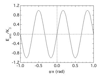
FIG. 2. In-plane trigonal anisotropy energy  $E_{\rm anis}$  normalized by the anisotropy constant  $K_3$  of a moment versus its angle  $\phi$  with respect to the positive x axis. The three minima of  $E_{\rm anis}$  are at  $\phi/\pi=-5/6,\ -1/6,\ {\rm and}\ 1/2.$
