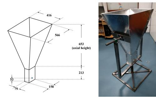
FIG. 16: Sketch of a simple Pyramidal horn with dimensions (in mm) and photograph of the fully fabricated antenna. The antenna is fed through an N-type coaxial connector and is mounted on an altitude-azimuth mount.
