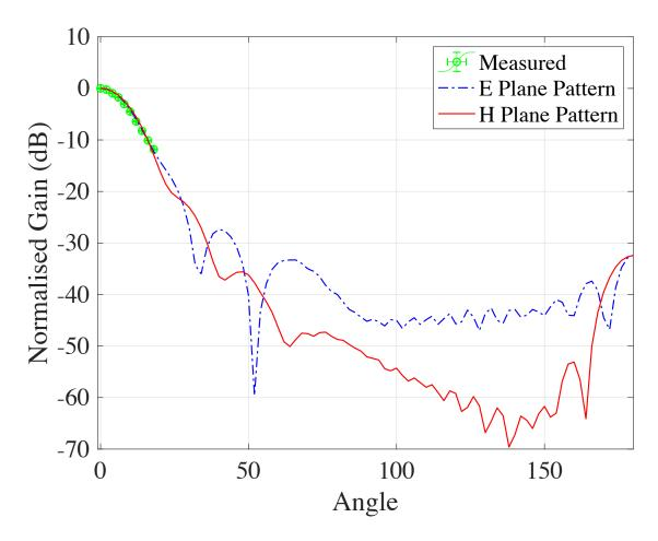
FIG. 4: Simulated and measured radiation patterns of the proposed horn. The worst sidelobe level is -27 dB in E-plane (blue curve). The measurement could only be done in E-plane due to limitations of the setup. The measured pattern is limited to -12 dB due to the sensitivity limitation of the setup.
