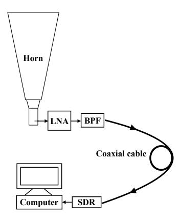
FIG. 5: Setup of the experiment. The low noise amplifier (LNA) and band pass filter (BPF) form the front-end electronics. A long, low-loss coaxial cable is used to connect the front-end to the back-end. Use of a long cable is recommended in order to avoid possible RFI generated by the computer. In the current setup, an LMR 400 cable is used. Other low-cost RF cables, e.g., RG58, with 50  $\Omega$  characteristic impedance, can also be used.
