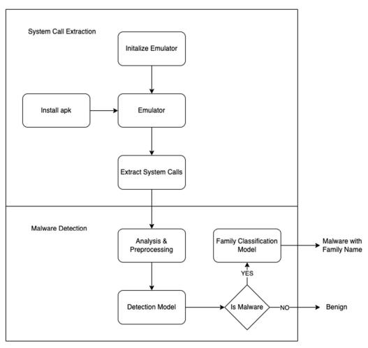
Fig 3.1 System Architecture of Malware Detection and Family Classification using System Calls
