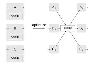
**Figure 2.** The common sub-computation comp replaces the three concurrent components A, B, and C.
