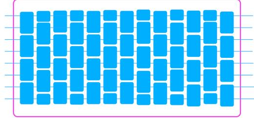
FIG. 1. Diagram showing a quantum circuit composed of single-qubit and two-qubit basic gates. Quantum circuit complexity quantifies the minimum number of basic gates needed to generate a target unitary.
