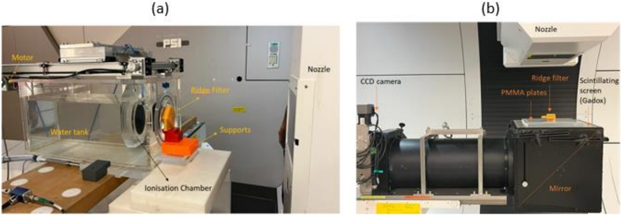
Figure 3 Experimental setup: (a) range scanner with RF placed closed to the isocenter, (b) CCD camera with PMMA plates and RF.
